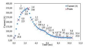
Figure 1. Fronius GMAW pulsed waveform.
