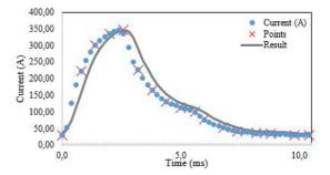
Figure 5. Result Fronius GMAW pulsed waveform.
