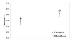
Figure 12. Weld pool temperature - Fronius and OTC Pulsed GMAW.
