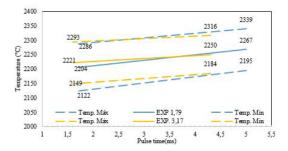
Figure 8. Droplet temperature versus pulse time.
