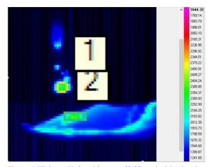
Figure 4. Highspeed infrared footage of [1] Detached droplets that fall into [2] weldpool without the luminous and thermal influence of the electric arc.
