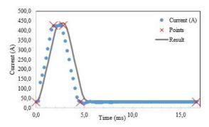
Figure 6. Result OTC GMAW pulsed waveform.
