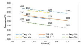
Figure 7. Droplet temperature versus Pulse current.
