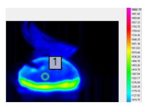
Figure 3. [1] Melted 309L-Si filmed for determination of his emissivity.
