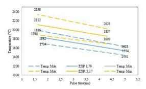
Figure 10. Weld pool temperature versus Pulse time.
