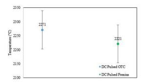
Figure 11. Droplet temperature - Fronius and OTC Pulsed GMAW.
