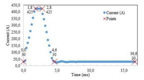
Figure 2. OTC GMAW DC pulsed waveform.
