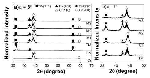
Figure 5. GAXRD patterns of as deposited coatings acquired with incidence angle of (a) 5° and (b) 1°.
