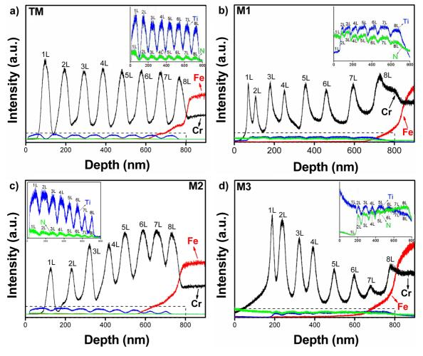
Figure 4. GD-OES profiles of TiN/Cr multilayers (a) TM, (b) M1, (c) M2 and (d) M3. Ti and N signals are evidenced in insets.
