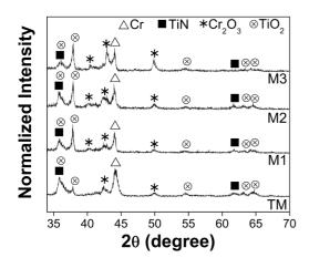
Figure 9. GAXRD patterns of coatings oxidized at 750°C.
