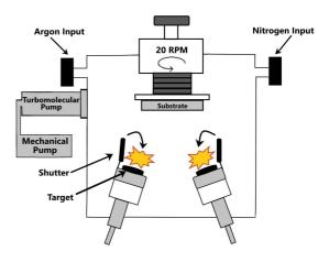
Figure 1. Schematic representation of deposition chamber.
