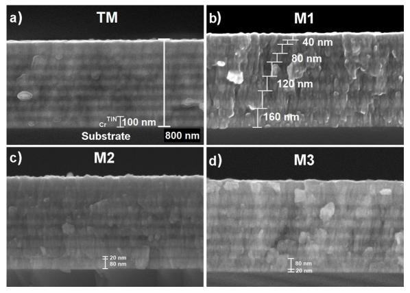
Figure 3. Micrographs of multilayers cross-sections (a) TM, (b) M1, (c) M2 and (d) M3 with magnification of 50000x.
