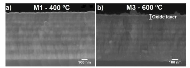
Figure 8. Cross-section SEM images with magnification of 50000x acquired after oxidation tests at (a) 400 °C and (b) 600 °C.
