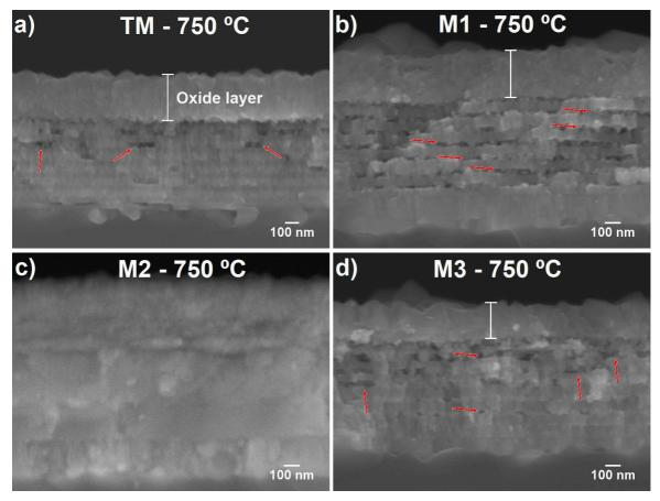
Figure 10. Cross-section SEM images with a magnification of 30000x acquired after oxidation tests at 750 °C.
