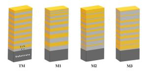
Figure 2. Schematic representation of multilayers architectures.
