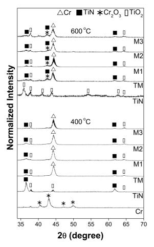
Figure 7. GAXRD patterns of coatings oxidized at 400 °C and 600 °C.
