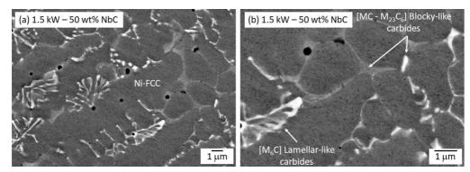
Figure 14. Interdendritic carbides formed in the coatings deposited with 1.5 kW laser power and 50% NbC feeding rate.
