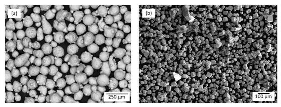
Figure 1. Typical feeding materials: Hastelloy C276<sup>™</sup> alloy (a) and Niobium Carbide (b).
