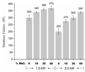
Figure 18. The hardness of composite coatings versus laser power and NbC feeding rate.
