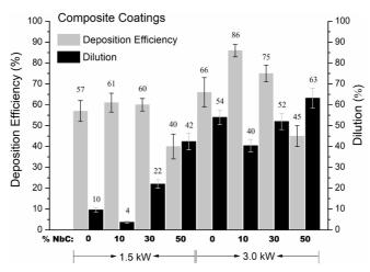
Figure 5. Average deposition efficiency and dilution.
