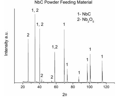
Figure 2. Typical X-ray patterns of NbC feeding powder.
