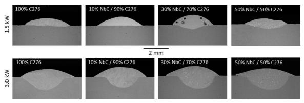
Figure 4. As deposited single-bead macrography of the coatings.
