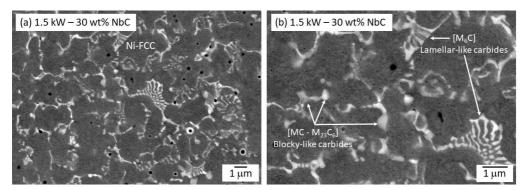
Figure 13. Interdendritic carbides formed in the coatings deposited with 1.5 kW laser power and 30% NbC feeding rate.
