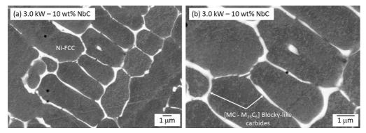
Figure 15. Interdendritic carbides formed in the coatings deposited applying 3.0 kW laser power and 10% NbC feeding rate.
