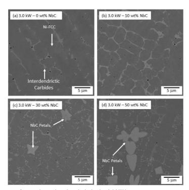
Figure 11. The microstructure of composite coatings deposited adopting 3.0 kW laser power.
