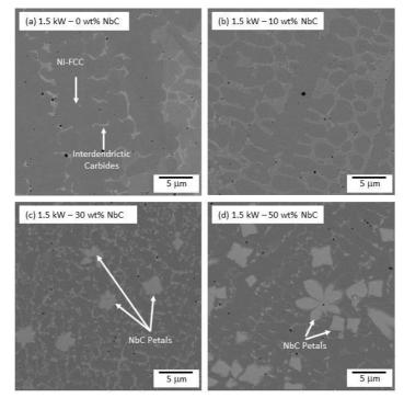
Figure 10. The microstructure of composite coatings deposited adopting 1.5 kW laser power.
