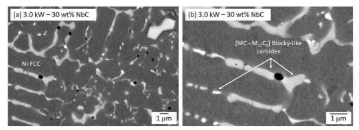
Figure 16. Interdendritic carbides formed in the coatings deposited with 3.0 kW laser power and 30% NbC feeding rate.
