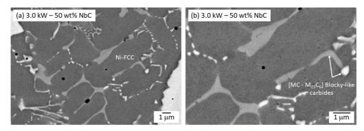
Figure 17. Interdendritic carbides formed in the coatings deposited with 3.0 kW laser power and 50% NbC feeding rate.
