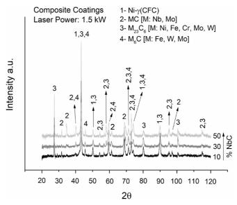
Figure 6. Typical X-ray diffraction pattern of composite coatings deposited applying 1.5 kW laser power.
