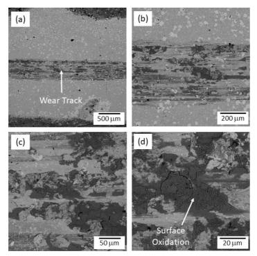
Figure 21. Wear track of the coating deposited with 1.5 kW and a 50% NbC feeding rate. Magnification increases from (a) to (d).
