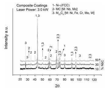
Figure 7. Typical X-ray diffraction pattern of composite coatings deposited adopting 3.0 kW laser power.
