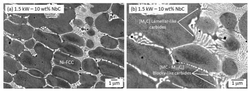
Figure 12. Interdendritic carbides formed in the coatings deposited with 1.5 kW laser power and 10% NbC feeding rate.
