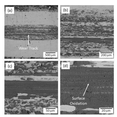
Figure 20. Wear track of the non-reinforced coating deposited with 1.5 kW. Magnification increases from (a) to (d).
