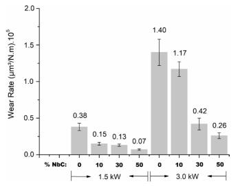
Figure 19. Wear rate of the composite coatings versus laser power and NbC feeding rate.
