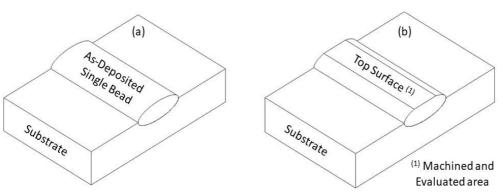
Figure 3. Schematic view of the single-bead: (a) as-deposited and (b) machined and evaluated top surface.
