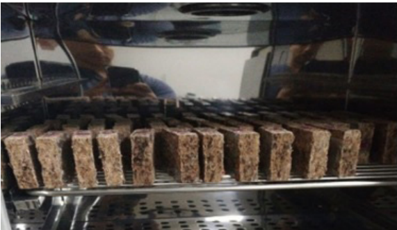
Figure 6. Aspects of specimens (a) Specimes at 100°C; (b) Specimes after 24 h at 100°C
