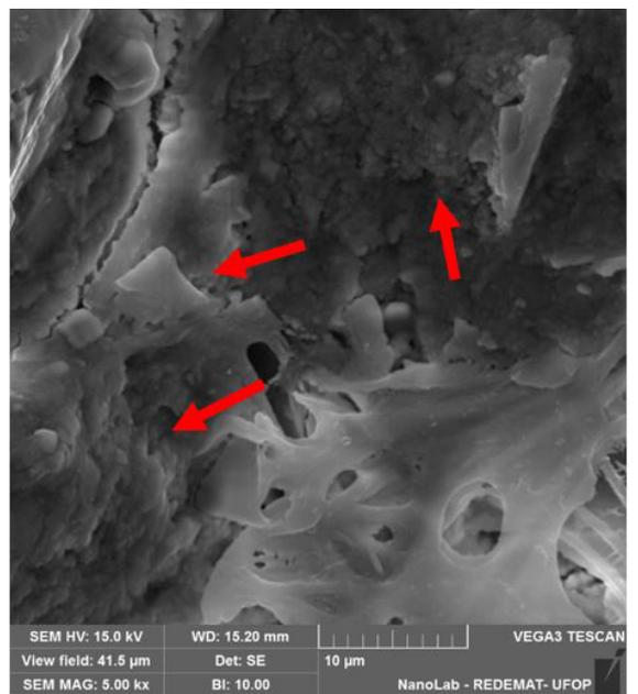
**Figure 8.** Micrograph of sample AF100-02 tested at 28 days with 5000x magnification.
