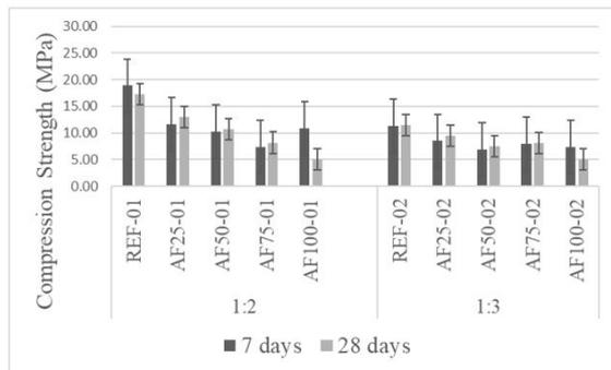
Figure 5. Compression Strength test results for 7 and 28 days.
