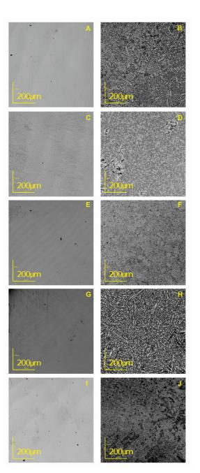
**Figure 3.** Representative micrographs of corrosion superficial. A) Co-Cr before Fusayama's saliva; B) Co-Cr after Fusayama's saliva; C) Co-Cr before Listerine® alcohol-containing; D) Co-Cr after Listerine® alcohol-containing; E) Co-Cr before Listerine® alcohol-free; F) Co-Cr after Listerine® alcohol-free; G) Co-Cr before Plax® alcohol-containing; H) Co-Cr after Plax® alcohol-containing; I) Co-Cr before Plax® alcohol-free.
