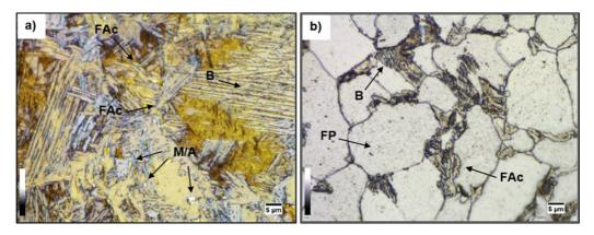
Figure 2. Quenching at 900 °C. (a) Acicular ferrite, elongated bainite plates and M/A in 160-Mo steel (Lepera - MOC); (b) polygonal ferrite, acicular ferrite and bainite in 056-Mo steel (Nital 2% - MOC).
