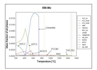
Figure 7. Thermodynamic simulation performed on steel 056-Mo: MC,  $M_3C_2$ ,  $M_7C_3$  and  $M_{23}C_6$  carbides.
