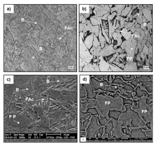
Figure 3. (a) and (c) 160-Mo after tempering at 450 and 600 °C. (b) and (d) 056-Mo after tempering at 450 and 600 °C (MOC and SEM – Nital 2%).
