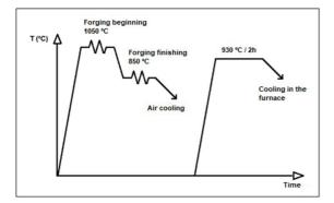
Figure 1. Thermomechanical processing of microalloyed steels.
