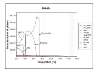
**Figure 6.** Thermodynamic simulation performed on steel 160-Mo: MC,  $M_4C_2$ ,  $M_7C_3$  and  $M_{23}C_6$  carbides.
