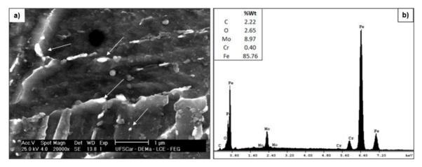
Figure 5. (a) and (b) Steel 160-Mo after quenching 900 °C and tempering 600 °C: particles of molybdenum carbides indicated by the arrows and the spectrum of concentrations obtained with the analysis by EDS (Nital 2% - SEM).
