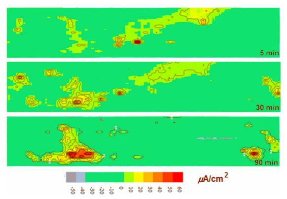
Figure 7. SVET ionic currents maps obtained for SAE 1008 carbon steel after 5, 30 and 90 minutes of immersion in 0.001 mol L<sup>-1</sup> HCl solution.
