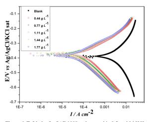
Figure 6. Tafel plot for SAE 1008 carbon steel in 0.5  $mol L^{-1}$  HCl solution in the absence and presence of different concentrations of cocoa bean shell powder.
