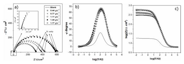
Figure 4. Nyquist (a) and Bode plots, for phase angle (b) and the logarithm of the impedance modulus (c) for carbon steel in the absence and presence of different concentrations of the cocoa bean shell powder in the  $0.5 \text{ mol } L^{-1}$  HCl solution.
