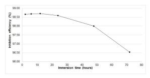
Figure 13. Corrosion inhibition efficiency at different immersion times in 0.5 mol  $L^{-1}$  HCl solution.
