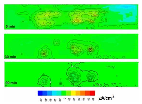
**Figure 8.** SVET ionic current maps obtained for SAE 1008 carbon steel after 5, 30 and 90 minutes of immersion in 0.001 0.5 *mol*  $L^{-1}$  HCl solution in the presence of 1.77 g  $L^{-1}$  inhibitor.
