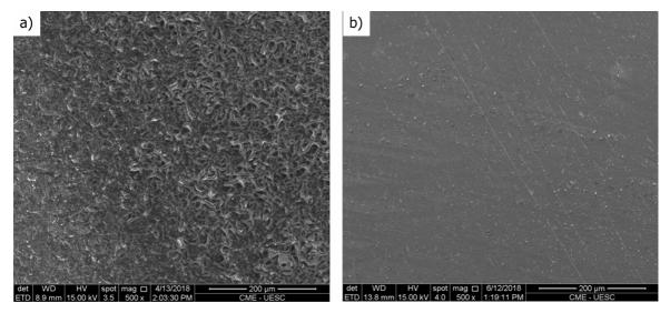
Figure 11. SEM micrographs of SAE 1008 carbon steel surface after immersion in the electrolyte, in the absence (a) and in the presence of inhibitor (b).
