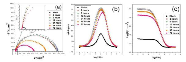
Figure 12. Nyquist (a) and Bode plots, containing the phase angle (b) and logarithm of the impedance modulus (c), for the carbon steel in the presence of  $1.77 \text{ g } L^{-1}$  of the cocoa bean shell powder at different immersion times.
