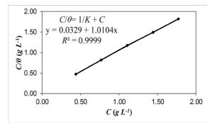
Figure 9. Langmuir adsorption isotherm for SAE 1008 carbon steel for different concentrations of cocoa bean shell powder in 0.5 mol L<sup>-1</sup> HCl.
