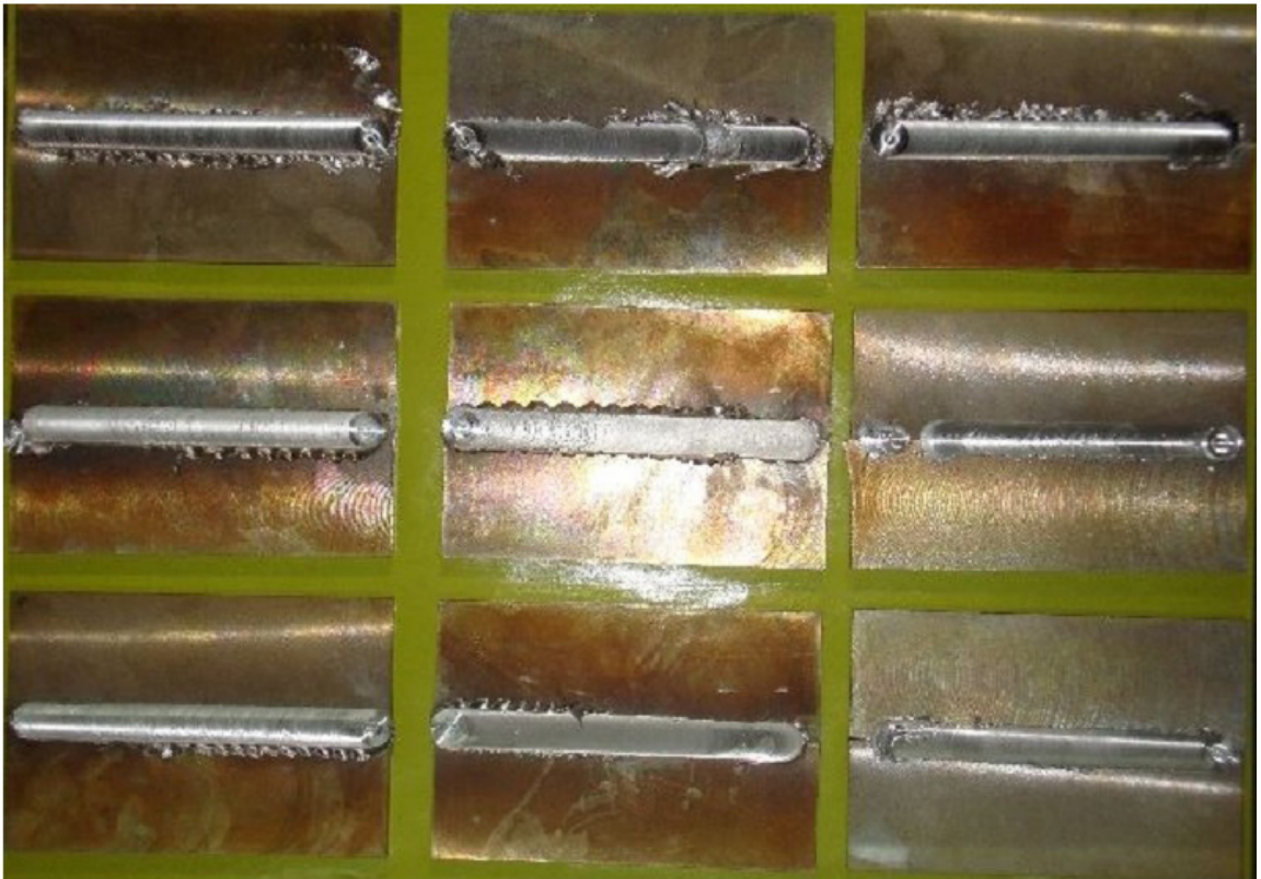
Figure 2. Photograph of some of the dissimilar FSWed AZ91C and AZ31B joint configuration fabricated during the 2 experimental sets.
