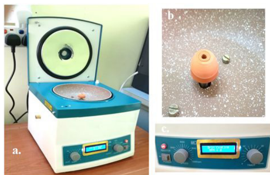
Figure 4. a. The final design of the spin coater, b. substrate holder, and c. front view of the spin coater speed controller.
