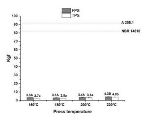
**Figure 9.** Face screw (FSP) and top (TSP) pull-out for particleboard panels produced with sugarcane bagasse and plastic bag particles at different pressing temperatures. \* Averages followed by a similar letter (uppercase for APF lower case for APT) did not differ statistically by the Scott-Knott test at 5% significance level.
