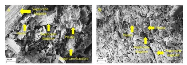
Figure 4. Images obtained by scanning electron microscopy for panels produced at 160°C (A) and 220°C (B).
