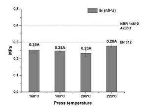
Figure 7. Internal bonding (IB) for particleboard panels produced with sugarcane bagasse and plastic bag particles at different pressing temperatures. \* Averages followed by similar letter did not differ statistically by the Scott-Knott test at 5% significance level.
