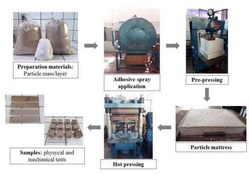
Figure 1. Production sequence of the particleboard.
