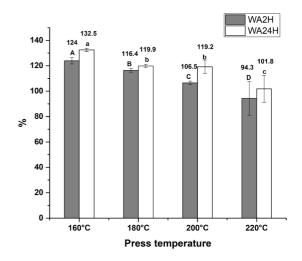
**Figure 2.** Water absorption for particleboard panels produced with sugarcane bagasse and plastic bag particles at different pressing temperatures. \*Averages followed by a similar letter (uppercase for WA2h and lower case for WA24h did not differ statistically by the Scott-Knott test at a 5% significance level.
