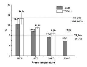
Figure 3. The swelling thickness of particleboard panels produced with sugarcane bagasse and plastic bag particles at different pressing temperatures. \*Averages followed by a similar letter (uppercase for TS2h and lower case for TS24h) did not differ statistically by the Scott-Knott test at a 5% significance level.
