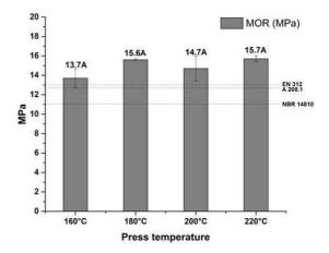
Figure 5. Modulus of rupture (MOR) for particleboard panels produced with sugarcane bagasse and plastic bag particles at different pressing temperatures. \* Averages followed by similar letter did not differ statistically by the Scott-Knott test at 5% significance level.
