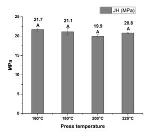
**Figure 8.** *Janka* hardness (JH) for particleboard panels produced with sugarcane bagasse and plastic bag particles at different pressing temperatures. \* Averages followed by similar letter did not differ statistically by the Scott-Knott test at 5% significance level.
