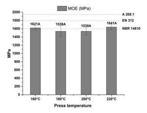
**Figure 6.** Modulus of elasticity (MOE) for particleboard panels produced with sugarcane bagasse particles at different pressing temperatures. \* Averages followed by similar letter did not differ statistically by the Scott-Knott test at 5% significance level.
