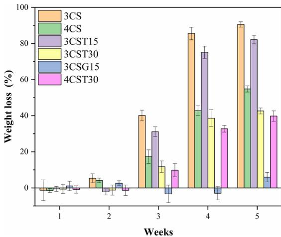
**Figure 9.** Mass variation of the CS woven meshes crosslinked with TPP and genipin at different times.
