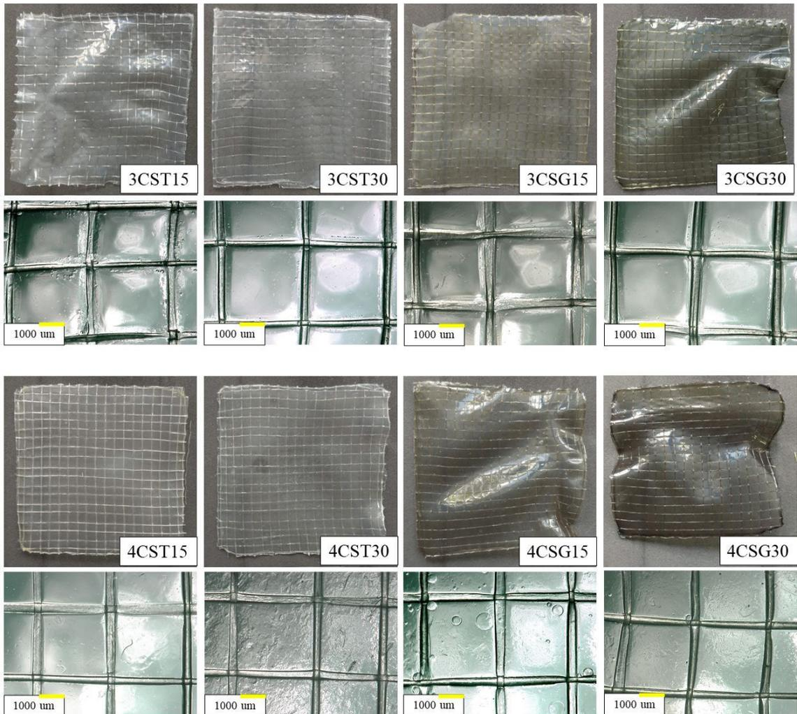
**Figure 4.** OM images of CS woven meshes crosslinked with TPP and genipin at different times.
