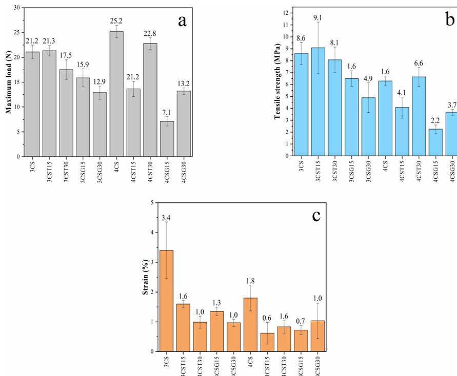
**Figure 5.** Mechanical properties of crosslinked and uncrosslinked CS woven meshes a) maximum load; b) tensile strength and c) strain.
