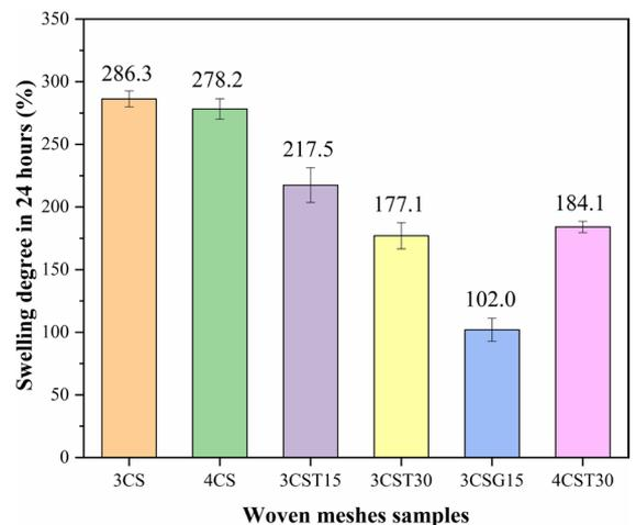
**Figure 7.** Swelling degree of CS woven meshes crosslinked with TPP and genipin at different times.
