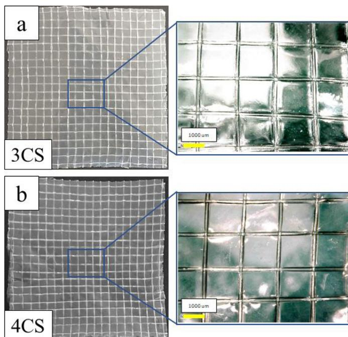
**Figure 3.** OM images of CS woven meshes. a) coated with 3% CS solution, b) coated with 4% CS solution.
