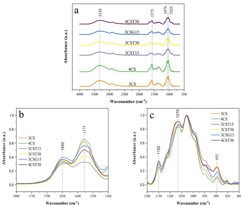
**Figure 6.** FT-IR spectra of crosslinked and uncrosslinked CS woven meshes a) from 4000 to 650 cm<sup>-1</sup>; b) from 1800 to 1500 cm<sup>-1</sup> and c) from 1200 to 800 cm<sup>-1</sup>.
