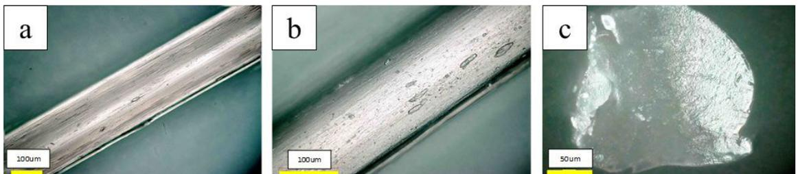
**Figure 2.** OM images of 4% CS filament obtained by wet spinning. Increases of a) 350x the longitudinal section, b) 700x the longitudinal section and c) 1050x the cross-section of the filament.
