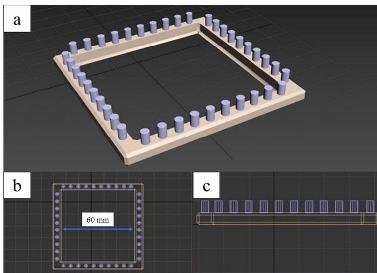
**Figure 1.** Views of the mold made by 3D printing for weaving of the CS meshes.
