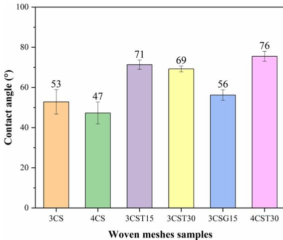
**Figure 8.** Contact angle of the CS woven meshes crosslinked with TPP and genipin at different times.
