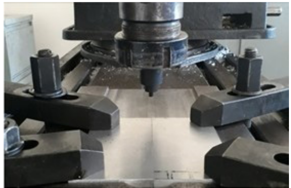
Figure 2. Fixing plates for welding execution.
