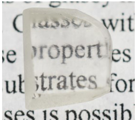
Figure 7. Sample 70GeO 2 ·10K 2 O·20Ta 2 O 5 with a central thickness of 4.8 mm treated at 840 °C for 48 h.
