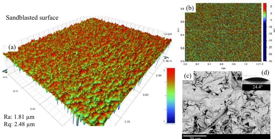
**Figure 2.** Optical profiling in 3D (a) and 2D (b), top-view SEM images (c), and a contact angle (d) of the sandblasted stainless-steel substrate uncoated.
