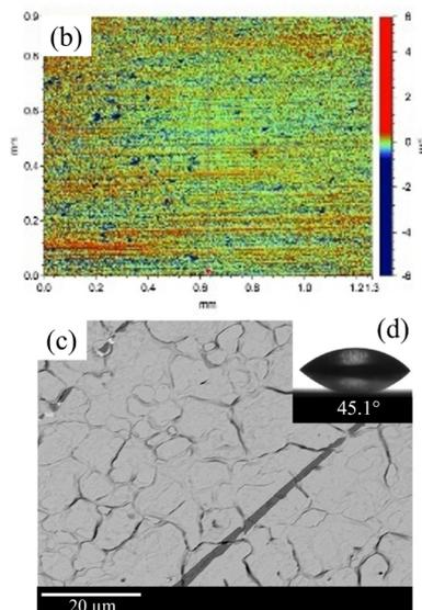
**Figure 1.** Optical profiling in 3D (a) and 2D (b), top-view SEM image (c), and a contact angle (d) of the smooth stainless-steel substrate uncoated.
