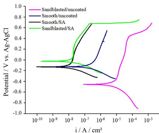
**Figure 6.** Polarization Curves of samples with smooth and sandblasted surface coated with SA compared with the uncoated samples analyzed in 0.1 mol / L of NaCl solution.
