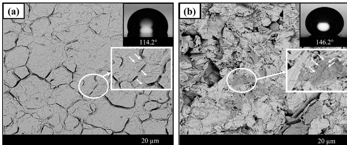
**Figure 3.** Top-view SEM micrographs and contact angle of the stainless-steel substrate with a smooth (a) and sandblasted surface (b) with a stearic acid (SA) coating.
