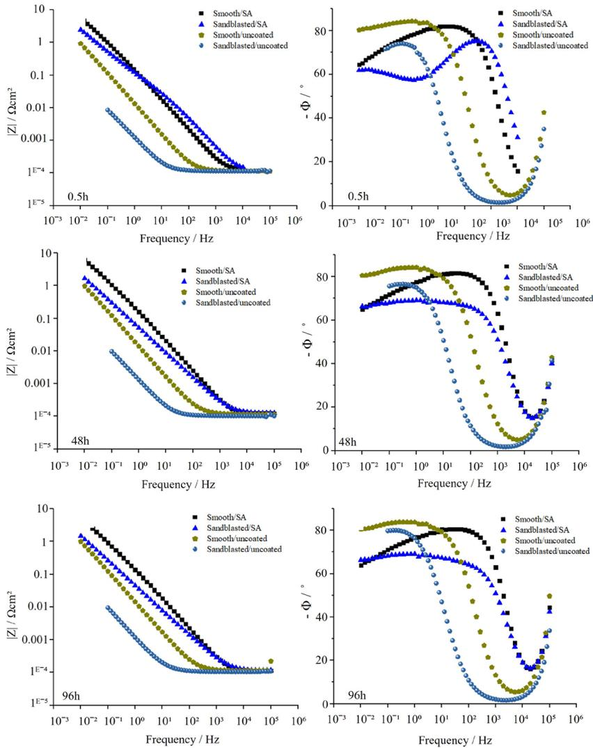
**Figure 5.** Bode diagrams of the samples with the smooth and sandblasted substrate with SA coating compared to the uncoated substrates analyzed in 0.5 h, 48 h, and 96 h of immersion in 0.1 mol / L NaCl solution.
