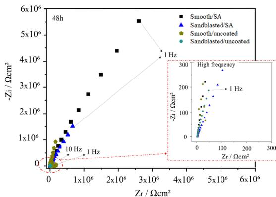
**Figure 4.** Nyquist diagram for smooth and sandblasted substrates with SA coating compared to the uncoated substrates, analyzed in 48 h of immersion in 0.1 mol / L NaCl solution.
