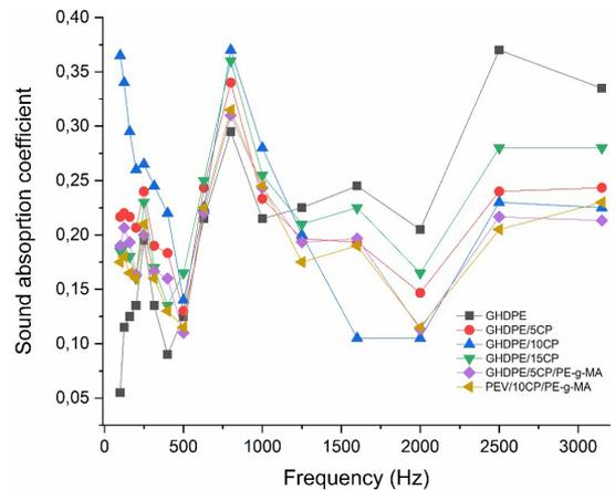
**Figure 4.** Acoustic absorption coefficient for GHDPE and its composites.
