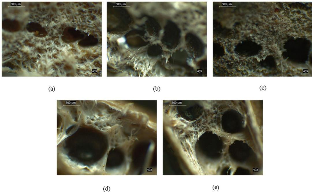
**Figure 5.** Optical microscopy of composites containing cork and compatibilizer: (a) GHDPE/5CP; (b) GHDPE/10CP; (c) GHDPE/15CP; (d) GHDPE/5CP/SPE-g-MA; (e) GHDPE/10CP/SPE-g-MA.
