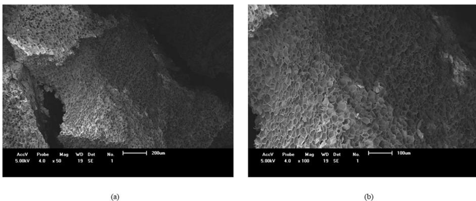
**Figure 6.** Morphological structure of cork: magnification 50x (a) and (b) 100x.
