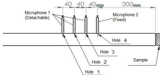
**Figure 1.** Microphone position in the impedance tube.
