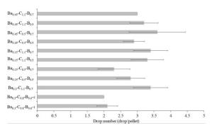
Figure 2. Influence of the composition on drop number of the green iron-ore pellets.
