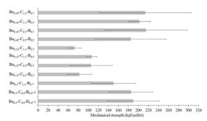
Figure 5. Influence of composition on the mechanical strength of the fired iron-ore pellets.
