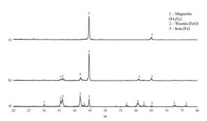
Figure 13. XRD spectra of the iron-ore pellets reduced in different isotherms: a) at the end of the 700  $^{\circ}$ C isotherm; b) at end of the 800  $^{\circ}$ C isotherm; and c) at the end of the reduction reaction.
