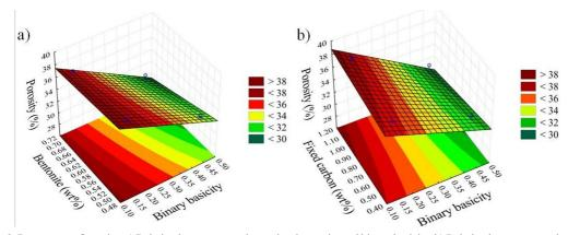
Figure 9. Response surface plot. a) Relation between porosity against bentonite and binary basicity. b) Relation between porosity against fixed carbon and binary basicity.
