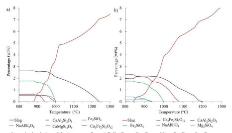
Figure 7. Thermodynamic simulation of the iron-ore pellets. a) Pellet  $Ba_{0.45}-C_{0.5}-B_{0.7}$  and b) pellet  $Ba_{0.3}-C_{1.1}-B_{0.7}$
