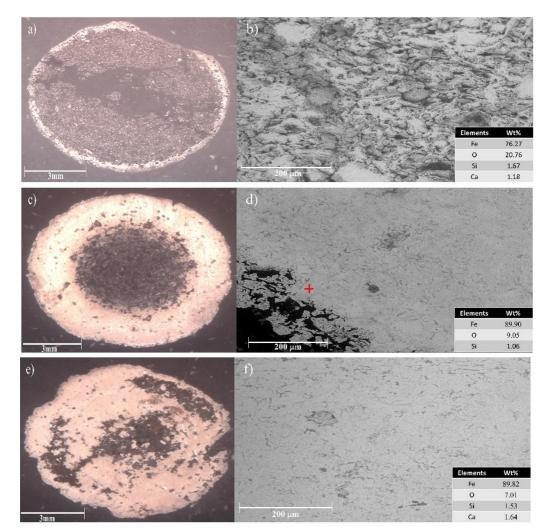
**Figure 12.** a) Optical microscopy at the end of the 700 °C isotherm; b) SEM image at the end of the 700 °C isotherm; c) optical microscopy image at the end of the 800 °C isotherm; d) SEM image at the end of the 800 °C isotherm; e) optical microscopy image at the end of the reduction reaction; and f) SEM image at the end of the reduction reaction.
