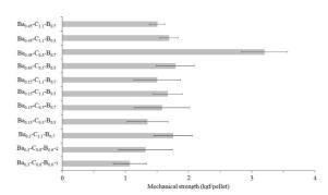
Figure 4. Influence of composition on the mechanical strength of the dried iron-ore pellets.
