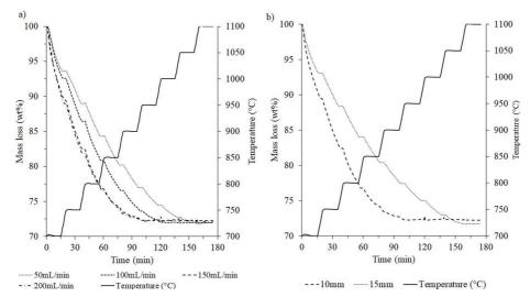
Figure 10. Thermogravimetric tests. a) Influence of CO flow on the reduction of the iron-ore pellet; b) influence of pellet diameter on the reduction reaction.
