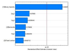
Figure 6. Pareto charts of the mechanical strength of the fired iron-ore pellets.
