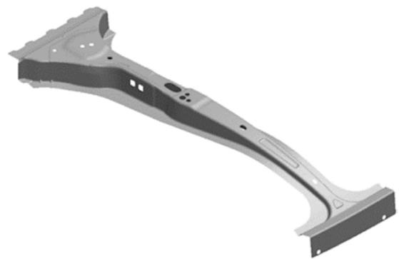
**Figure 2.** CAD drawing of the B-pillar workpiece.
