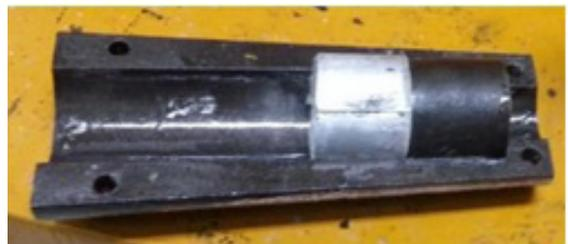
Figure 1. Cold compressed billet before extrusion.
