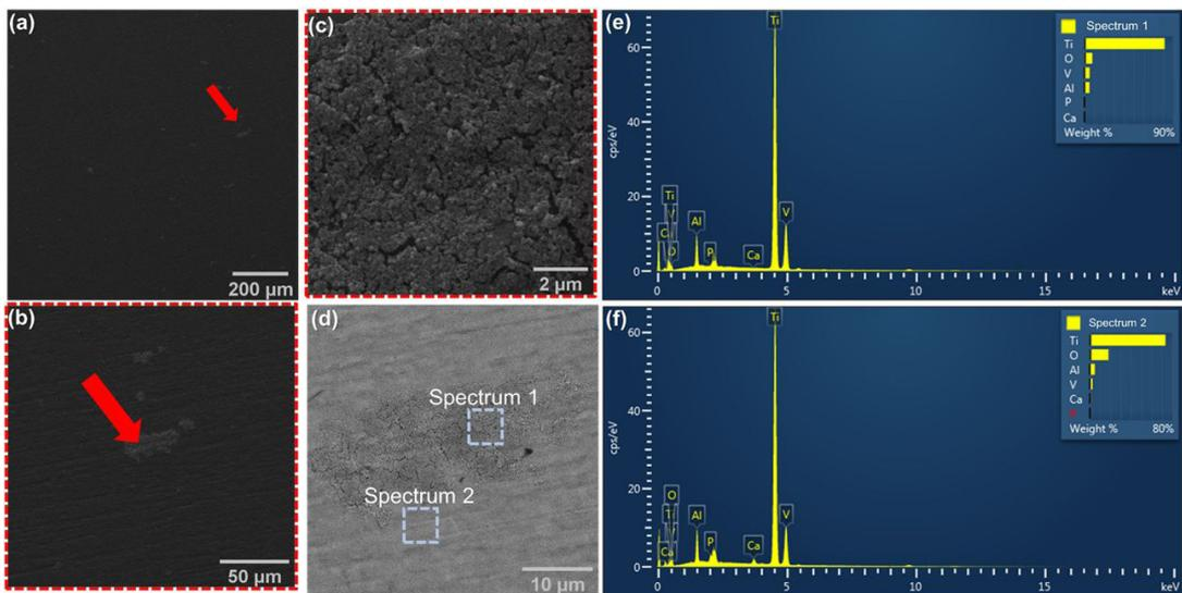
**Figure 8.** Analysis via SEM/EDX of the uncoated Ti-6Al-4V titanium alloy surface. (a) micrograph acquired using SE mode, (b) the region indicated in (a) at a higher magnification, (c) micrograph obtained via BSE of the region indicated in (b), (d) micrograph obtained via SE, and (e, f) show a spectra of two regions highlighted in (d).
