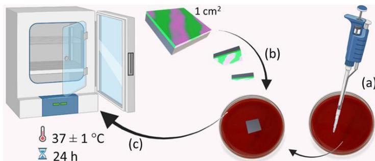
**Figure 1.** Representative drawing showing the steps for the inhibition halo assay. (a) The *S. aureus* suspension, adjusted to 0.5 on the McFarland scale was transferred to the blood agar culture medium, (b) the samples were placed in the culture with the evaluated surfaces facing downwards and (c) the plates were incubated for a period of 24 h at a temperature of  $37 \pm 1$  °C.
