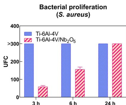
**Figure 6.** Count of Colony Forming Units (CFU) of *S. aureus* in direct contact with the Ti-6Al-4V alloy surface (used as negative control) and in contact with the coated Ti-6Al-4V/Nb<sub>2</sub>O<sub>5</sub> alloy surface. In the positive control there was no bacterial proliferation, therefore the results are not shown.
