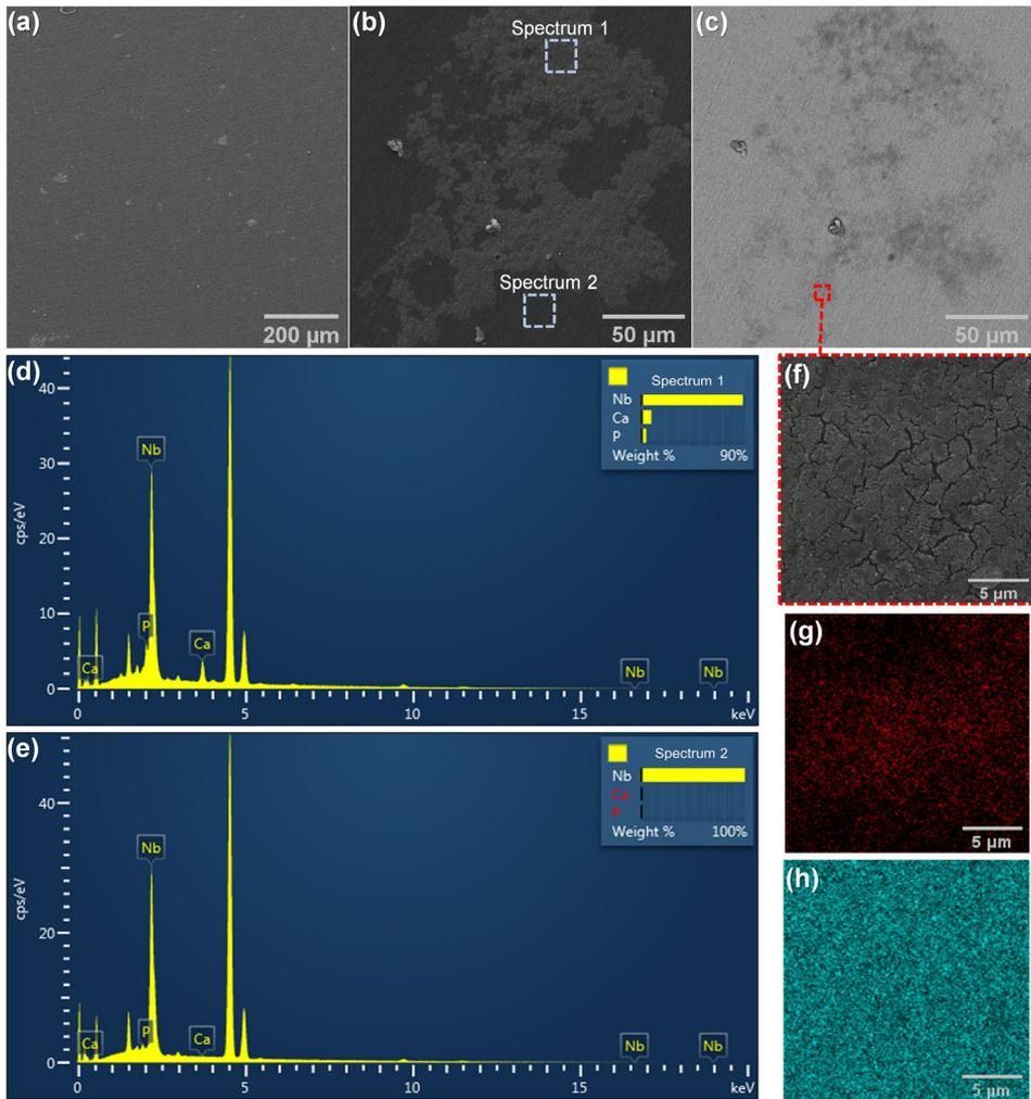
**Figure 9.** Analysis via SEM/EDX of the Ti-6Al-4V/Nb<sub>2</sub>O<sub>5</sub> titanium alloy surface. (a, b) micrograph obtained via SE and (c) BSE mode, (d, e) spectra of two regions of the analyzed sample's surface. (f) region highlighted in (c) obtained via SE mode at a higher magnification, (g, h) maps obtained via EDX to assess the presence of Ca and P, respectively.
