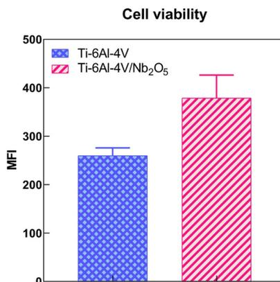
**Figure 3.** Cell Viability of MC3T3 Cells grown on the evaluated surfaces: Ti-6Al-4V (used as negative control) and Ti-6Al-4V/Nb<sub>2</sub>O<sub>5</sub> (given by the Mean Fluorescence Intensity - MFI).
