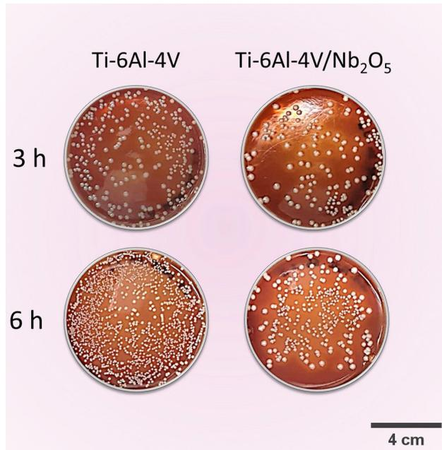
**Figure 7.** Qualitative result of *S. aureus* incubated at  $37 \pm 1$  °C for 24 h after direct contact for 3 and 6 h with the Ti-6Al-4V alloy surface and in contact with the coated Ti-6Al-4V/Nb<sub>2</sub>O<sub>5</sub> alloy surface. In the positive control there was no bacterial proliferation, therefore the results are not shown.
