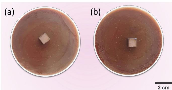
**Figure 5.** Plates with bacterial culture for 24 h in contact (a) with the uncoated Ti-6Al-4V alloy surface and (b) in contact with the coated Ti-6Al-4V alloy surface.
