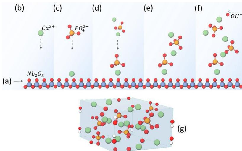
**Figure 10.** Simplified schematic model proposed to understand the nucleation mechanism of hydroxyapatite on the Ti-6Al-4V alloy surface containing Nb<sub>2</sub>O<sub>5</sub> thin films.
