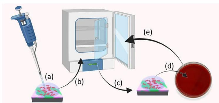
**Figure 2.** Schematic drawing showing steps for assaying antibacterial activity through direct contact assay. (a) bacterial suspension was added together with 200  $\mu$ L of Brain Heart Infusion Broth on the studied samples' surfaces and (b) incubated at a temperature of  $37 \pm 1$  °C. (c and d) After 3, 6, 24 and 48 h, 10  $\mu$ L of this culture were removed and inoculated onto blood agar plates, (e) which were then incubated at  $37 \pm 1$  °C for 24 h.
