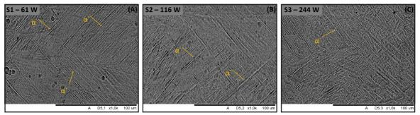
Figure 1. Micrographs of the L-PBF specimens presenting acicular martensite  $\alpha$ ' and some pores for lack of fusion. A) 61 W. b) 116 W and c) 244 W. Kroll reagent, 15 min, room temperature. SEM – BSE detector.
