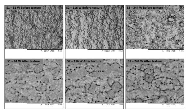
Figure 2. (A) Sample 1, built using 61 W, before and after texture; (B) Sample 2, built using 116 W, before and after texture; (C) Sample 1, built using 244 W, before and after texture.
