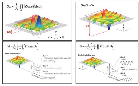
Figure 6. Schematic drawing about the parameters Sa, Sz, Ssk and Sku.<sup>26</sup>
