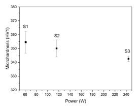
Figure 4. Microhardness values, obtained to Sample 1, 2 and 3, built using, respectively, 61 W, 116 W and 244 W.
