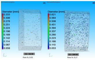
Figure 3. 3D porosity by x-ray tomography analysis. (a) Sample 1, built using 61 W; (b) Sample 2, built using 244 W.
