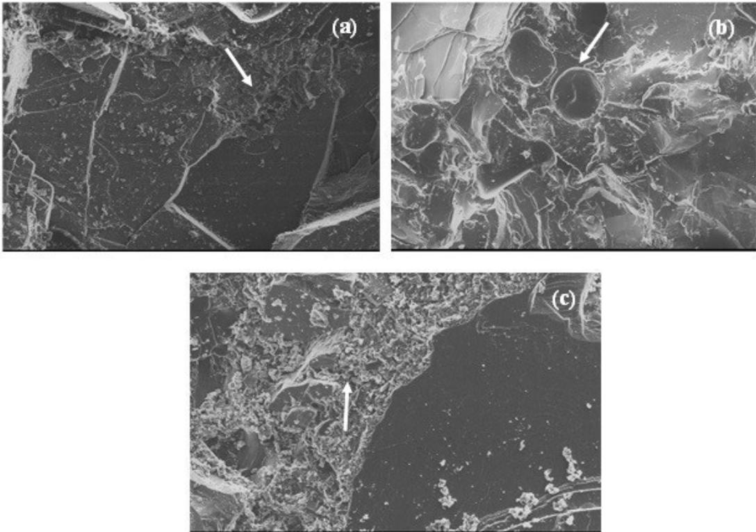
**Figure 3.** SEM of the fractured surface sections of artificial stone with granite and quartzite residue and epoxy resin as binder, ASGQ-5 (a), ASGQ-7 (b) and ASGQ-8 (c) at 100x magnification.
