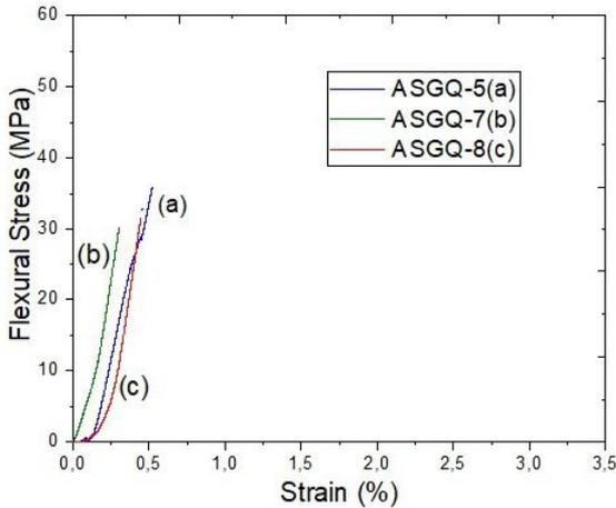
**Figure 4.** Mechanical behavior in the 3-point bending test, after the wetting and drying test: Artificial stone with granite and quartzite residue and epoxy resin as binder ASGQ-5 (a), ASGQ-7 (b) and ASGQ-8 (c).
