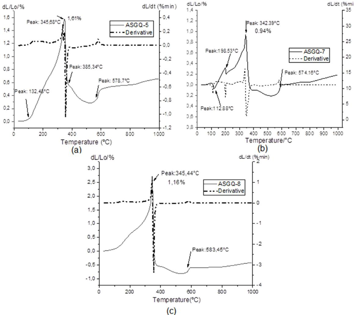
**Figure 5.** Dilatometer and curve derived from artificial stone with quartzite and quarry gravel residue (ASGQ), in compositions 5, 7 and 8. ASGQ-5 (a), ASGQ-7 (b) and ASGQ-8 (c).
