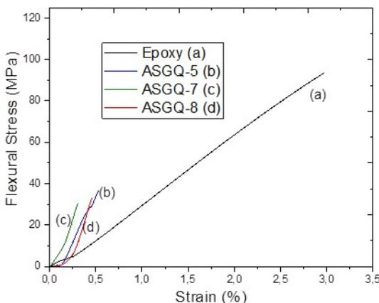
**Figure 2.** Mechanical behavior in 3-point bend test for Epoxy (a), and for artificial stone with granite and quartzite residue with epoxy resin, ASGQ-5 (b), ASGQ-7 (c) and ASGQ-8 (d).
