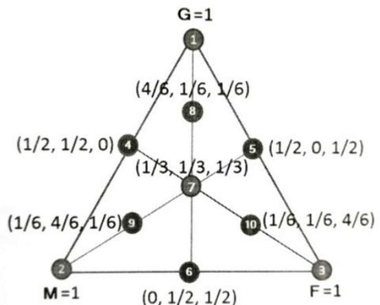
**Figure 1.** Ternary diagram with the 10 mixtures based on the Simplex-Lattice Design grid. Amounts (wt%) of Large (L), Medium (M) and Fine (F) particles.
