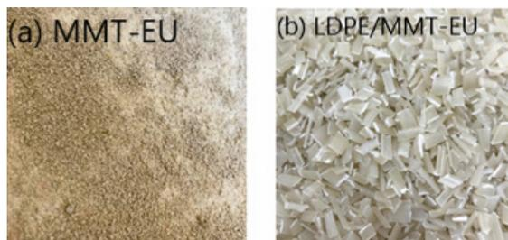
**Figure 1.** (a) montmorillonite-erucamide nanocomposite (MMT-EU) produced with 15 wt% of montmorillonite (Cloisite 20A) and with 85 wt% of erucamide – magnification of 20 times. (b) masterbatch (LDPE/MMT-EU) produced with 85 wt% of LDPE and with 15 wt% of MMT-EU nanocomposite - magnification of 10 times.
