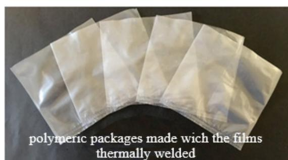
**Figure 2.** Polymeric packages made with the films thermally welded. Example: for the composition LLDPE with 10 wt% of LDPE/MMT-EU.
