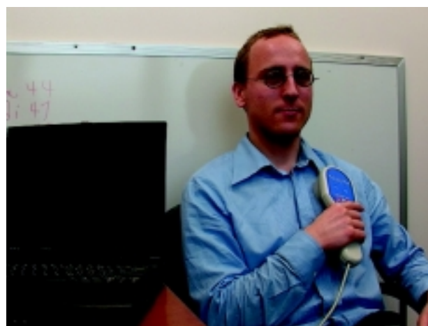
Figure 3 - Application of Vagus Nerve Stimulation: The NCP ® Programming Wand and a portable computer provide telemetric communication with the pulse generator, which enables noninvasive programming, functional assessments, and data retrieval.
