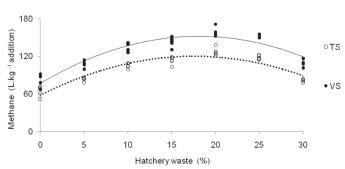
**Figure 4** – Methane specific production as a function of TS and VS addition to substratesconsisting of cattle manure and increasing liquid hatchery waste levels.
