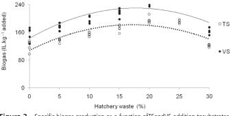
**Figure 2** – Specific biogas production as a function ofTSandVS addition tosubstratesconsisting of cattle manure and increasing liquid hatchery waste levels.
