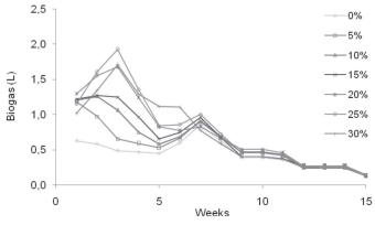
**Figure 3** – Time distribution of biogas production by substratesconsisting of cattle manure and increasing liquid hatchery waste levels.
