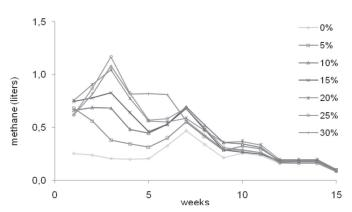
Figure 5 – Time distribution of methane production by substrates consisting of cattle manure and increasing liquid hatchery waste levels
