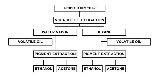
Figure 1. Flow diagram for the production of flavour free oleoresin.
