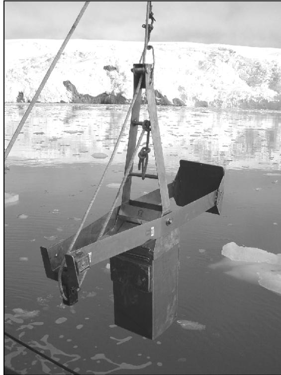
**Figure 2** - Mini Box Corer GEAMB ready for deployment.
