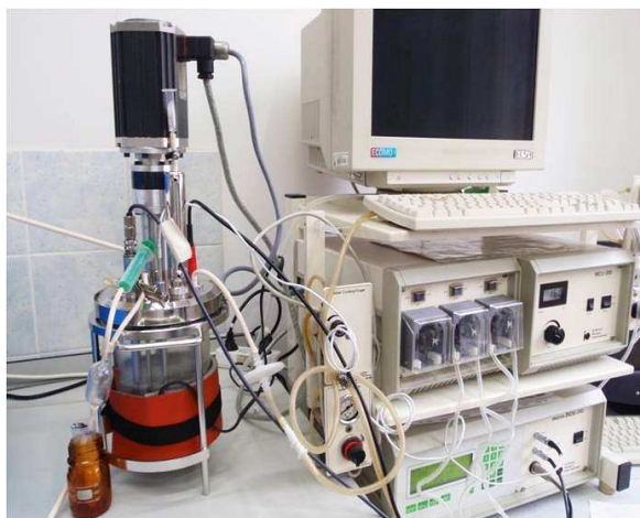
Figure 1 - Picture of the bioreactor.
