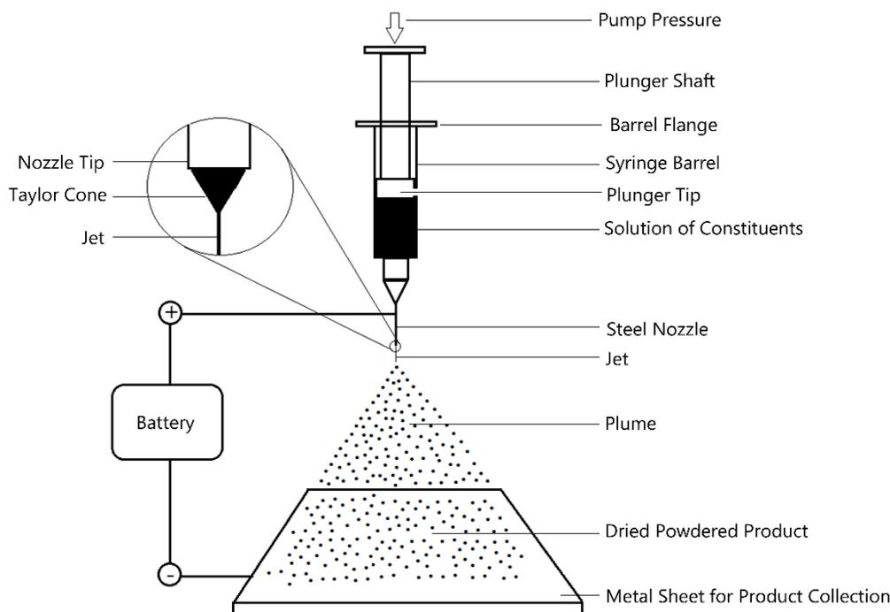
**Figure 2.** Schematic illustration of the electrospaying equipment.
