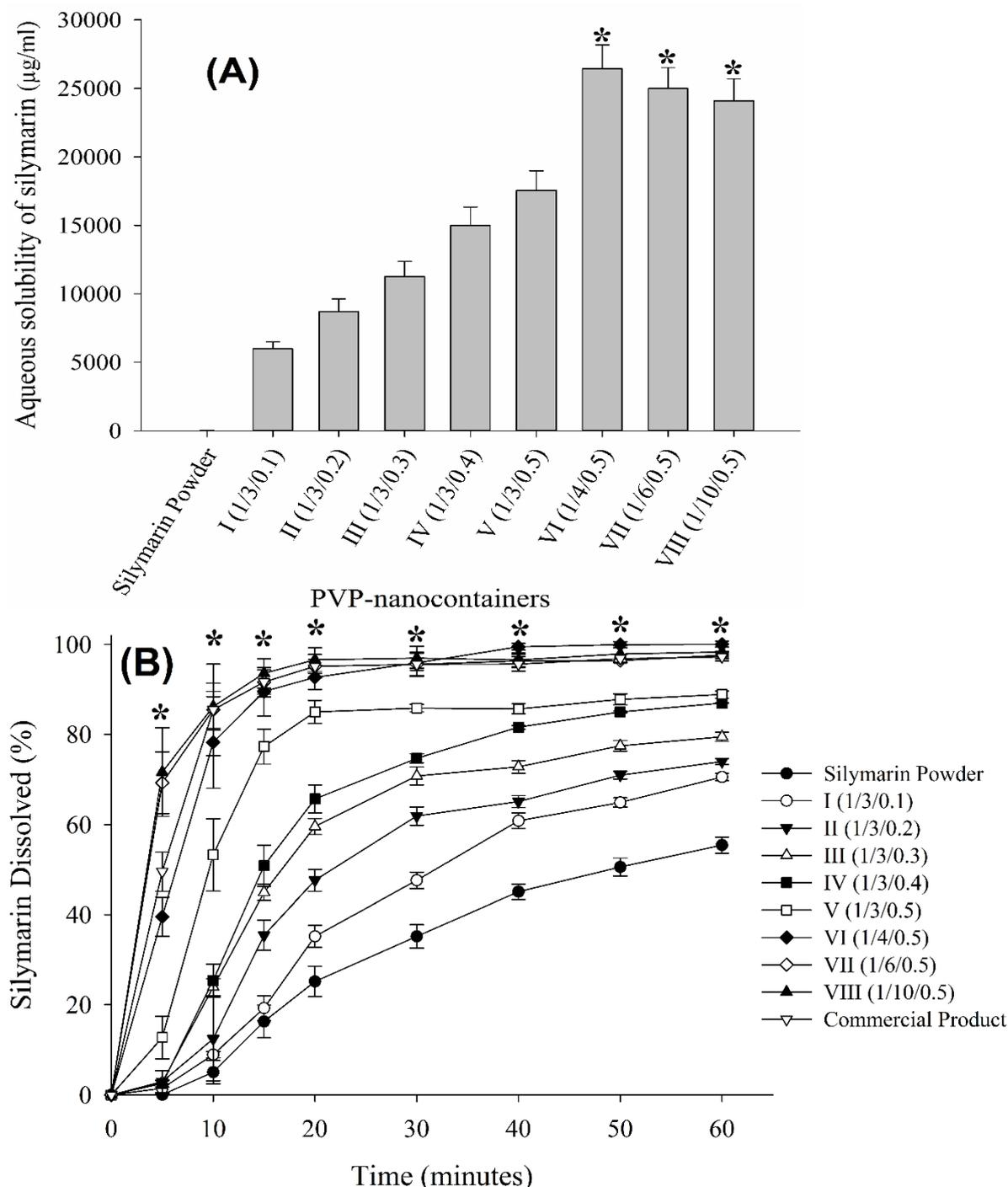
**Figure 3.** Effect of SDS (I-V) and PVP (VI-VIII) on the aqueous solubility (A) and the dissolution rate (B) of silymarin in the electrospayed nanocontainers. Each value of solubility and dissolution rate denotes the mean  $\pm$  S.D. ( $n = 3$  and  $6$ , respectively). \* $p < 0.05$  compared with the silymarin plain powder and formulations I-V.
