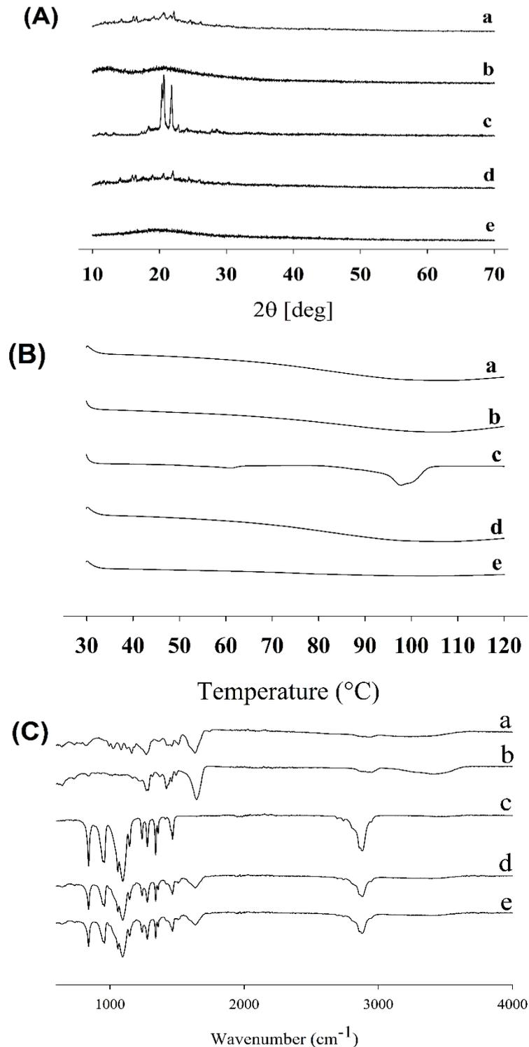
**Figure 5.** PXRD patterns (A); DSC thermograms (B); FTIR spectra (C): (a), silymarin plain powder; (b), PVP; (c), SDS; (d), physical mixture; (e) silymarin-laden PVP-nanocontainer formulation VI.
