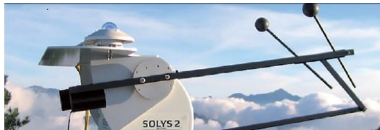
Figure 8. Solar Tracker from Kipp&Zonen , model Solys2 .
