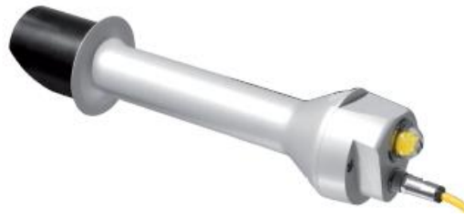
Figure 6. Pырheliometer from Kipp&Zonen , model CHP1 .
