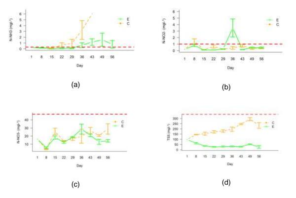
**Figure 9.** Weekly values of the control - C (n=4) and experimental - E (n=4) treatment of: (a) N-NH<sub>3</sub><sup>-</sup>; (b) N-NO<sub>2</sub><sup>-</sup>; (c) N-NO<sub>3</sub><sup>-</sup>; (d) TSS. Recommended values for shrimp culture are shown in the dashed red line.
