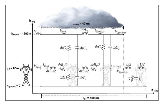
**Figure 1.** Model of local atmospheric electric circuit coupling with a transmission line. In this representation, there are capacitances, inductances, resistances and inductances between the ground and the storm cloud. The considered length of the transmission line is 500km and the storm cloud is about 1500m from the ground. Source: The authors (2021).
