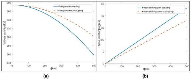
**Figure 3.** (a) Correlation between transmission line voltage with and without atmospheric coupling in respect to z (no losses). (b) Phase shifting in respect to distance (no losses) ~14%. The authors (2021).
