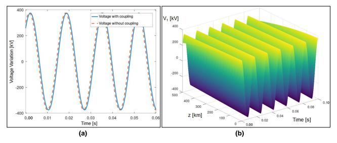
**Figure 2.** (a) Transmission line voltage in respect to time and space. (b) Comparison curves between transmission line voltages with and without atmospheric coupling effect, z = 500km (no losses). The authors (2021).
