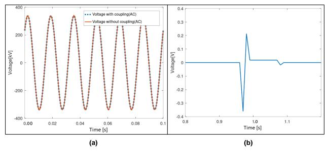
**Figure 6.** (a) Transmission line voltage correlation with and without atmospheric coupling considering the AC component (z=500km). (b) Indirect induced transmission line voltage due to an atmospheric cloud to ground discharge. The authors (2021).
