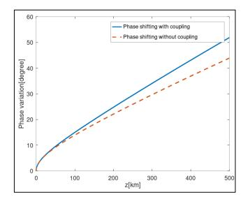
Figure 5. Phase shift in relation to distance, considering losses in a 375kV transmission line. The authors (2021).
