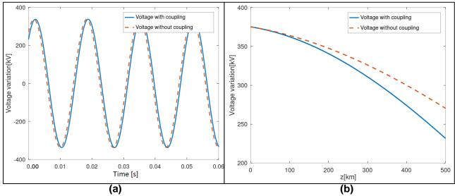
**Figure 4.** (a) Transmission line voltage with and without atmospheric coupling, considering losses (z = 500km). (b) Voltage magnitude with respect to distance, considering losses. Considering the atmospheric coupling, the voltage drop accumulated along the transmission line is more relevant than in the case of no coupling. The authors (2021).
