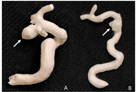
**Figure 7.** Aneurysm models made of PLA material. (A) Aneurysm located in the C7 segment of the ICA, measuring 2.8 x 7.6 mm. (B) ACI C4 segment aneurysm, measuring 4.5 x 6 mm.
