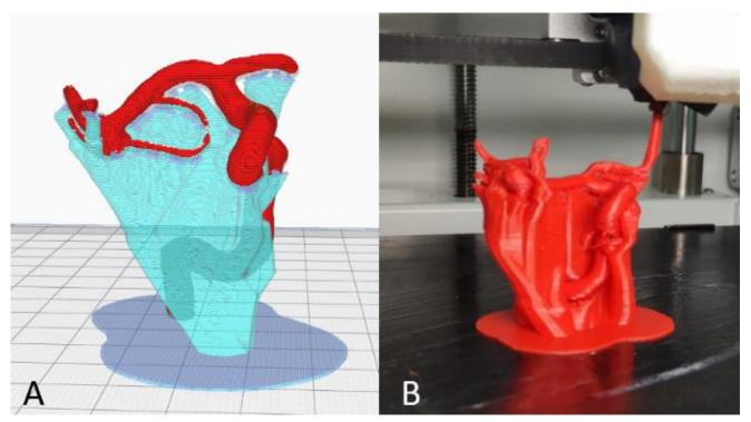
Figure 5. (A) The model in the Cura® software, ready for printing, and (B) the model being printed.
