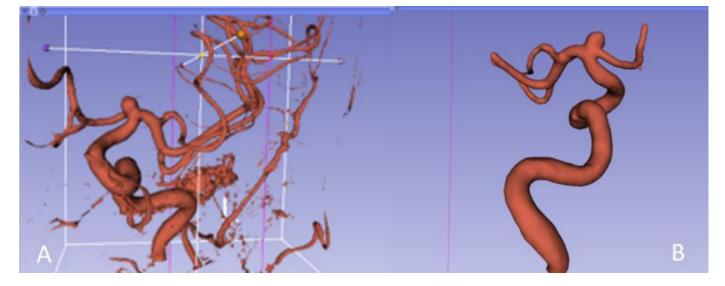
Figure 4. (A) The Generation of the form of the mask. (B) 3D model after cleaning the areas that are not needed. This is the final file, which will be sent to the Ultimaker Cura® software for AM.
