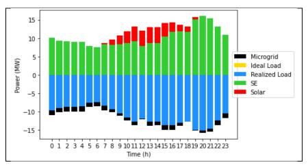
Figure 5. Power balance indexes of the feeder for the planning horizon with the distributed energy resources used.
