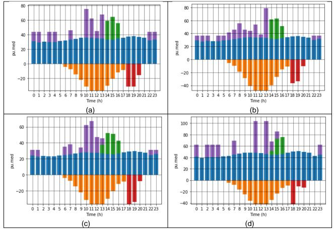
**Figure 1.** MOuG optimization dispatch during pre-processing for microgrids (a) 1, (b) 2, (c) 3, and (d) 4. NC-load in blue; C-load in purble, battery charge in green; battery discharge in red; PV-gen in red.
