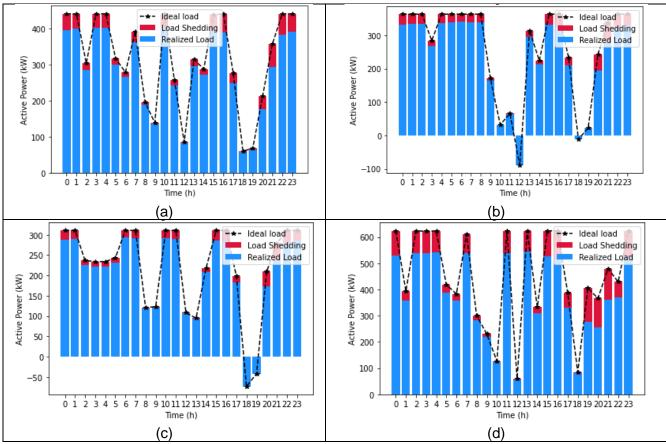
Figure 7. Ideal power injection from the main grid point of view for microgrids (a) 1; (b) 2; (c) 3; and (d) 4.
