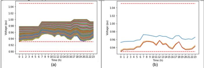
Figure 4. (a) Voltage for all buses; (b) Voltage for GLD buses.
