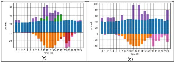
Figure 8. MOuG optimization dispatch in case III for microgrids (a) 1, (b) 2, (c) 3, and (d) 4. NC-load in blue; C-load in purple, battery charge in green; battery discharge in red; PV-gen in red.
