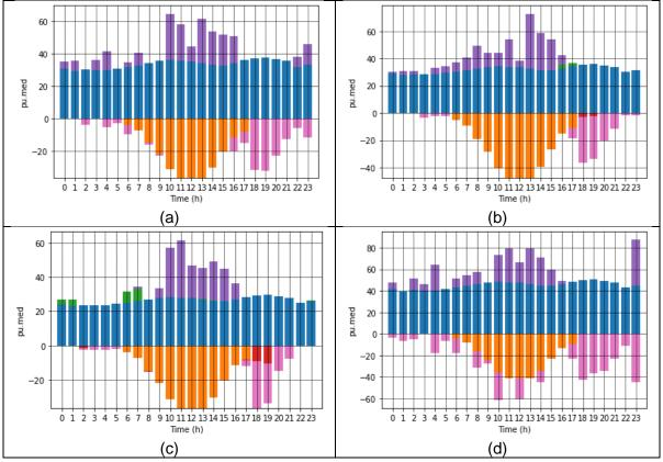
**Figure 3.** MOuG optimization dispatch in case II for microgrids (a) 1, (b) 2, (c) 3, and (d) 4. NC-load in blue; C-load in purble, battery charge in green; battery discharge in red; PV-gen in red.
