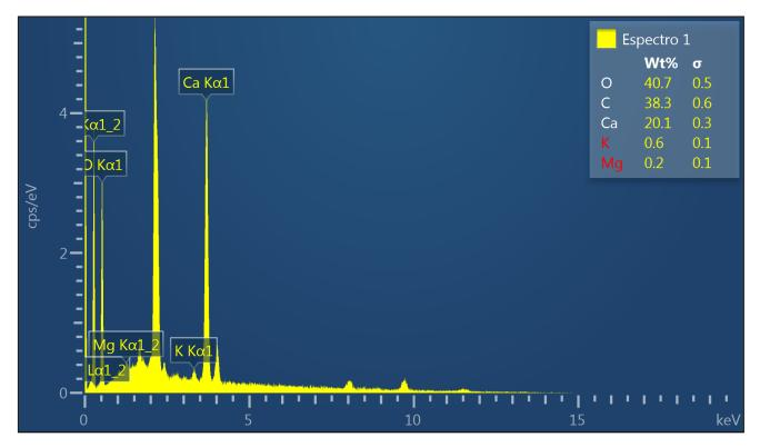
Figure 3. Energy-dispersive X-ray Spectroscopy (EDS) spectrum of prismatic crystal from Acmella bellidioides.
