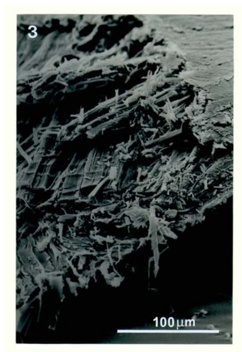
Figure 3: Scanning electron micrograph of the ground powder: membrane showing layers and bundles of pseudoboehmite fibrils.
