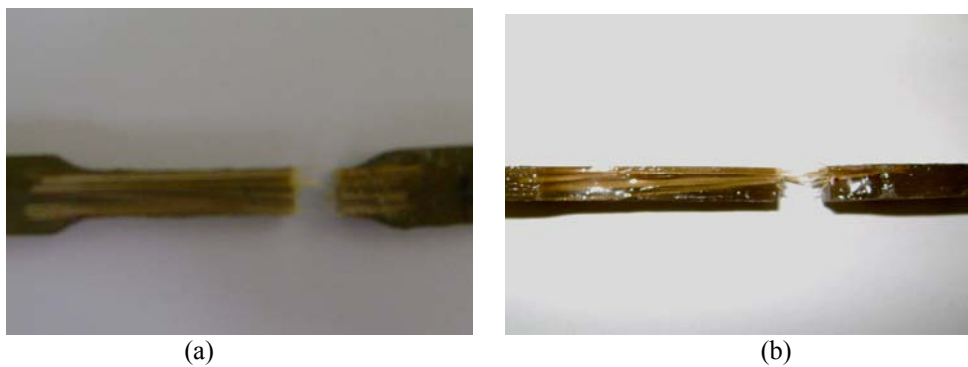
Figure 6: Macroscopic aspect of the ruptured tip of a polyester composite specimen reinforced with 40% of thinner buriti petiole fibers. (a) front view; (b) side view.
