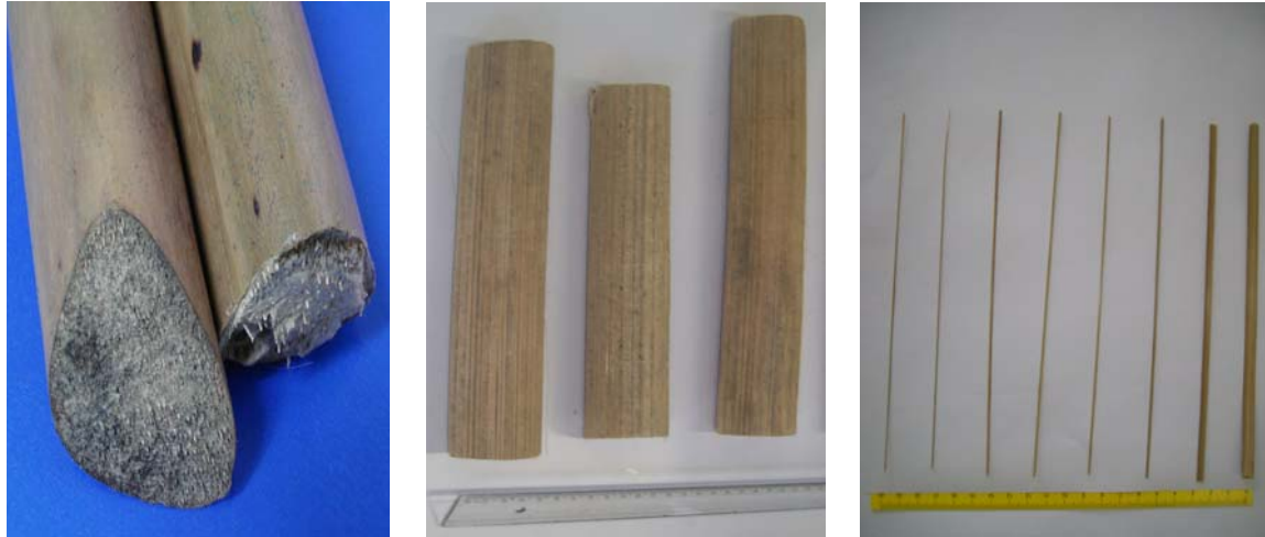
Figure 1: Buriti petioles and their fibers used in this investigation.
