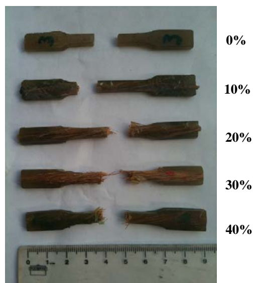
Figure 3: Representative tensile ruptured specimens for each volume fraction of coir fiber in polyester composites.
