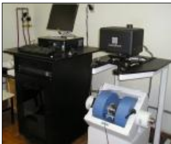
Figure 4: Magnetometer of Vibrant Sample name Lake Shore, Model 7410.
