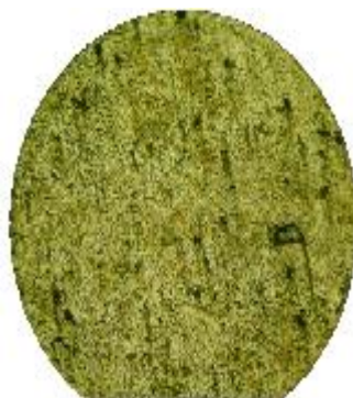
Figure 2: Etching nital 4%; magnification 160x.
