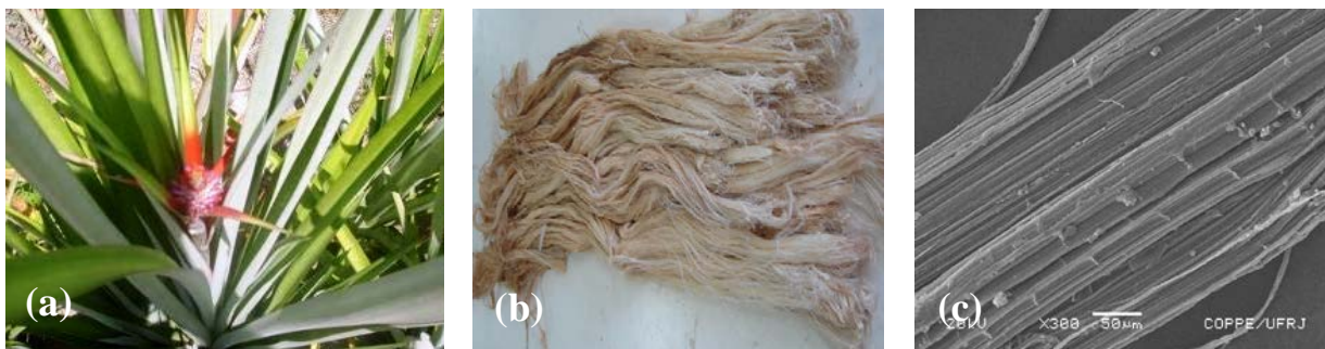
Figure 1: Curaua plant (a), bundle of fibers (b) and fibrils observed by scanning electron microscopy (c).
