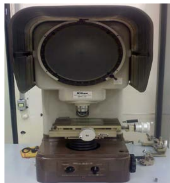
Figure 3: Profile projector Nikon used to measure the diameters of the curaua fibers.
