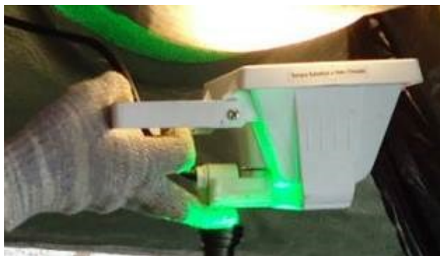
Figure 2: Halogen lamp used for thermal loading.
