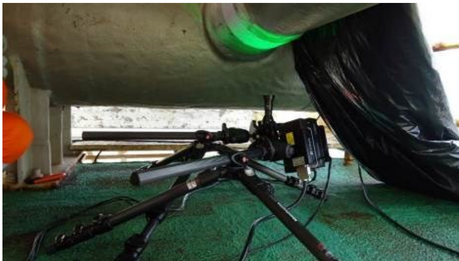
Figure 5: Shearography inspection at a composite repair in an offshore platform. The carbon fiber tripod can be observed.
