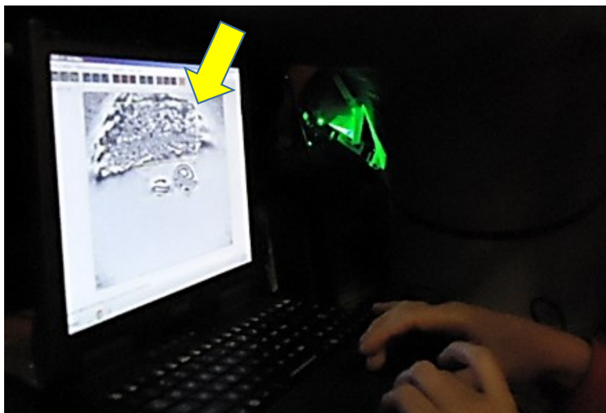
Figure 9: Shearography system control and data processing: visualization of a flawed region (arrow) in a composite repair.
