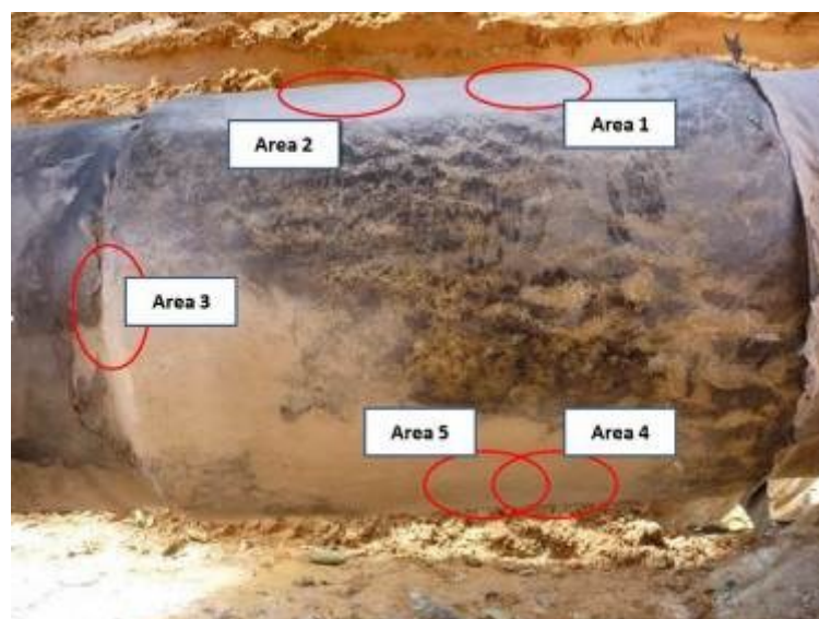
Figure 3: Regions measured with shearography system.
