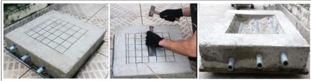
Figure 8: Cutting into the concrete body to evaluate the galvanized tubes.
