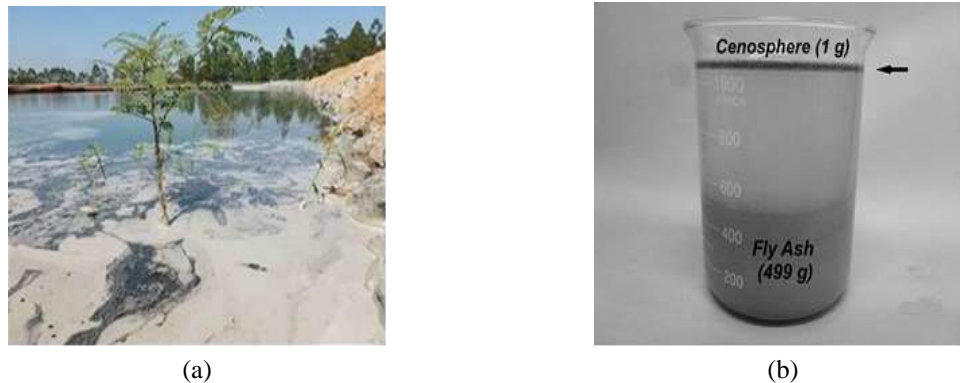
Figure 2: (a) View of the cenosphere-containing fly ash effluent decantation deposit showing the cenosphere-rich floating material. (b) The separation of cenosphere from the fly ash. The cenosphere is the floating layer and the fly ash is at the bottom of the Becker.
