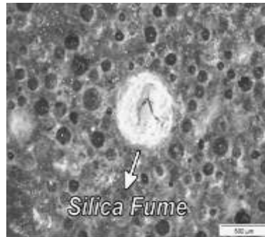
Figure 6: Silica fume agglomerate not adequately mixed to the matrix of a HP100 specimen.
