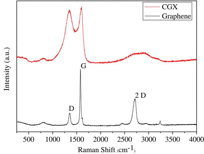
**Figure 2:** Raman spectra of CGX and graphene samples.
