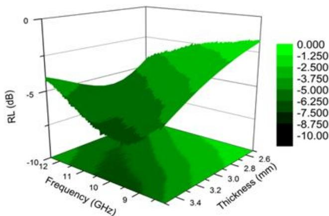
**Figure 7:** 3D Reflection Loss graph for sample 6 based on thickness variation.
