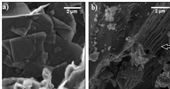
**Figure 1:** SEM picture of graphene (a), 30.0 kx and SEM picture of CGX (b).
