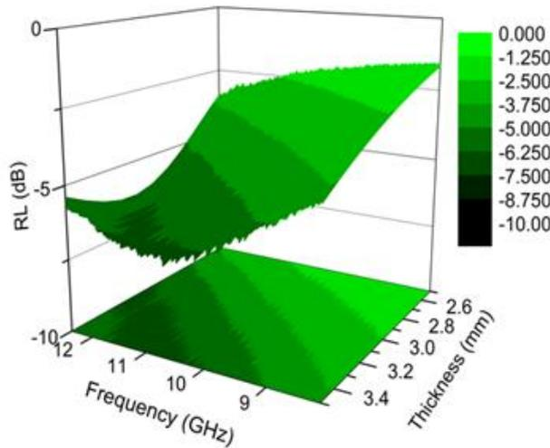
Figure 6: 3D Reflection Loss graph for sample 5 based on thickness variation.
