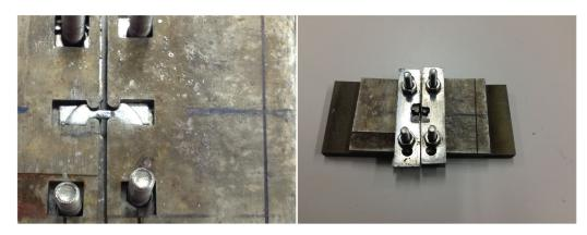
Figure 3: The clamping mould in tensile test.
