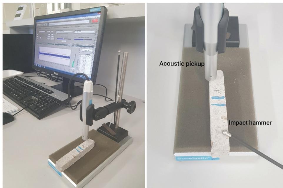
**Figure 1:** Sample in the elastic modulus tester.
