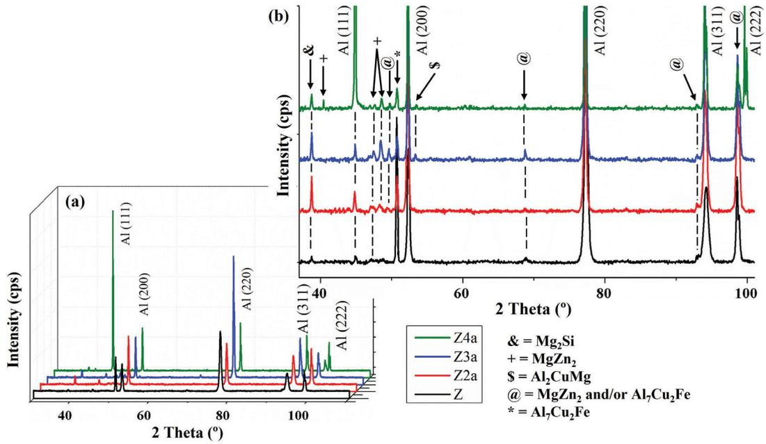
Figure 4: XRD patterns of Z, Z2a, Z3a and Z4a samples. (a) General aspect and (b) highlighting the precipitated peaks.
