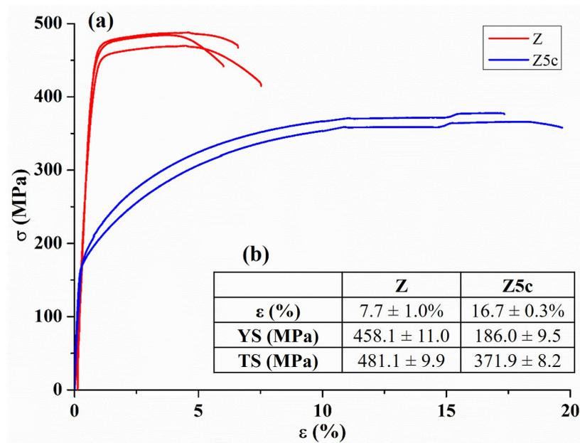
**Figure 8:** (a) Engineering Stress – Strain curves ( $\sigma$  (MPa) x  $\epsilon$  (%)) for Z and Z5c samples. (b) Average and standard deviations values of YS, TS and  $\epsilon$ .
