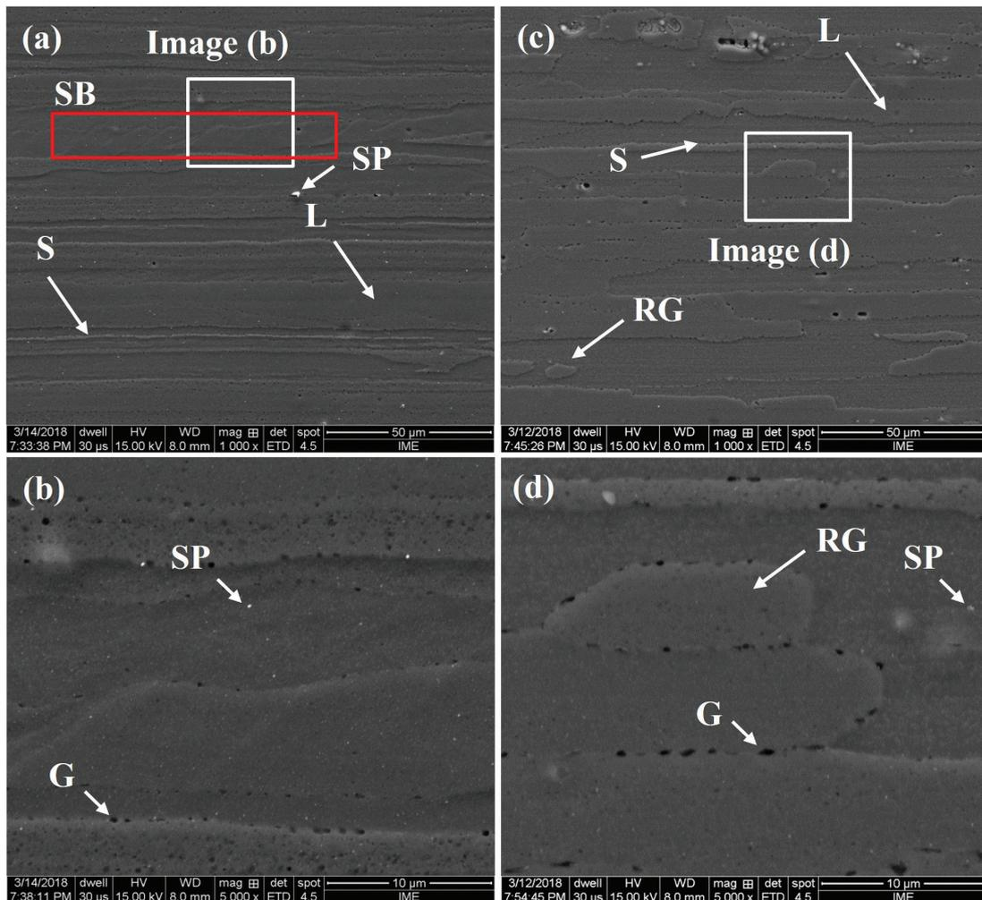
**Figure 6:** Microstructure of Z ((a) and (b)) and Z5c ((c) and (d)) samples visualized by SEM with lower magnification ((a) and (c)) and higher magnification ((b) and (d)).
