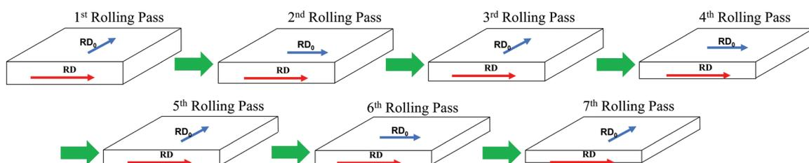
Figure 1: Sequence of passes performed in the present work for cross-rolling.
