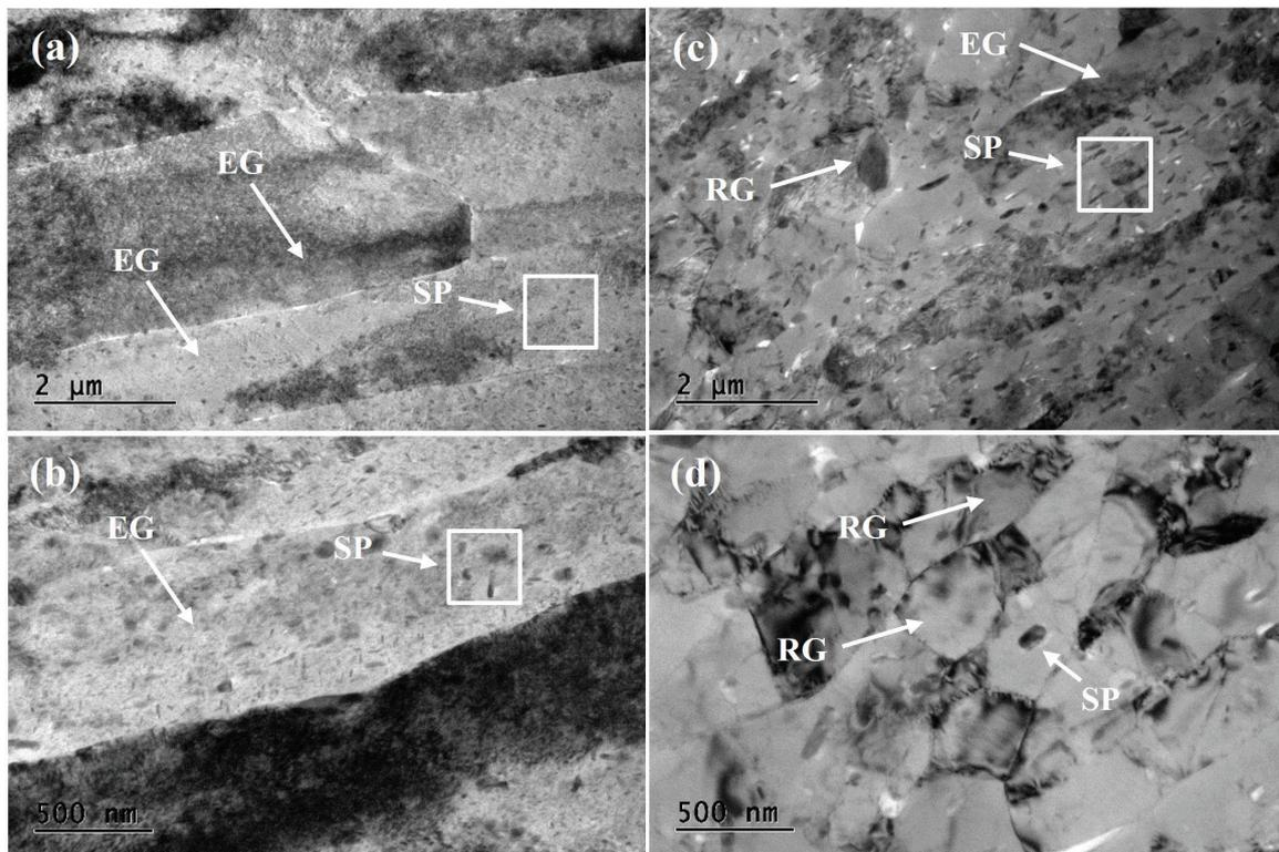
**Figure 7:** Microstructure of Z ((a) and (b)) and Z5c ((c) and (d)) samples visualized by TEM with lower ((a) and (c)) and higher ((b) and (d)) magnification.
