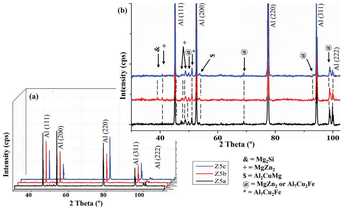
Figure 5: XRD patterns of Z5a, Z5b and Z5c samples. (a) General aspect and (b) highlighting the precipitated peaks.
