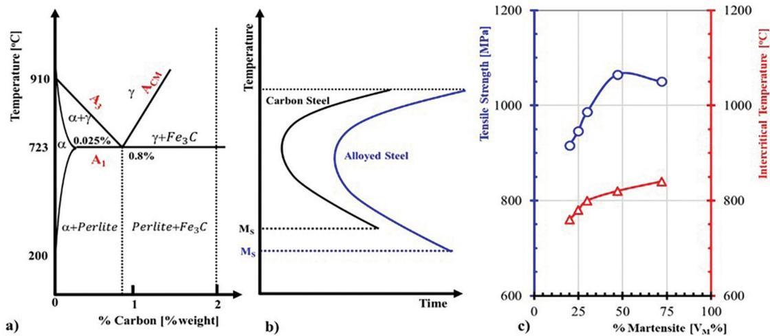
**Figure 2:** Fe-C diagrams in a), TTT in b), and correction of martensite volume, intercritical temperature, and mechanical strength in c).
