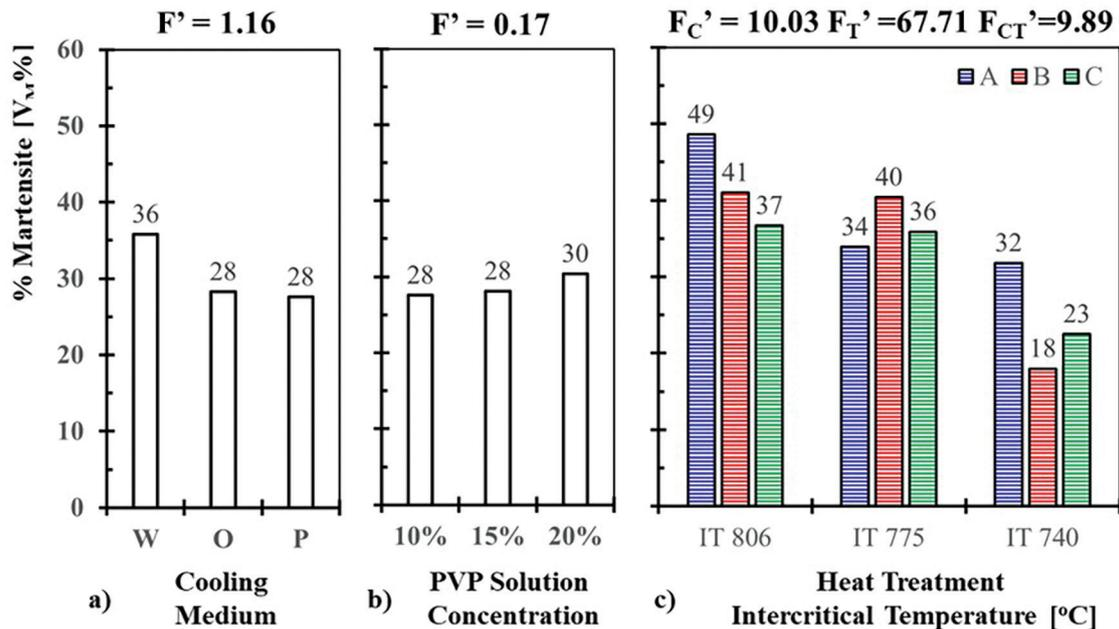
Figure 6: Martensite fraction derivate from intercritical heat treatment of HSLA samples (Dual Phase Steel).
