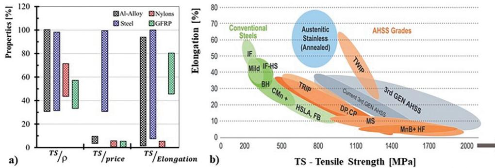
**Figure 1:** Comparison of mechanical properties for different materials (a) and different generations of steel developed in recent decades (b).
