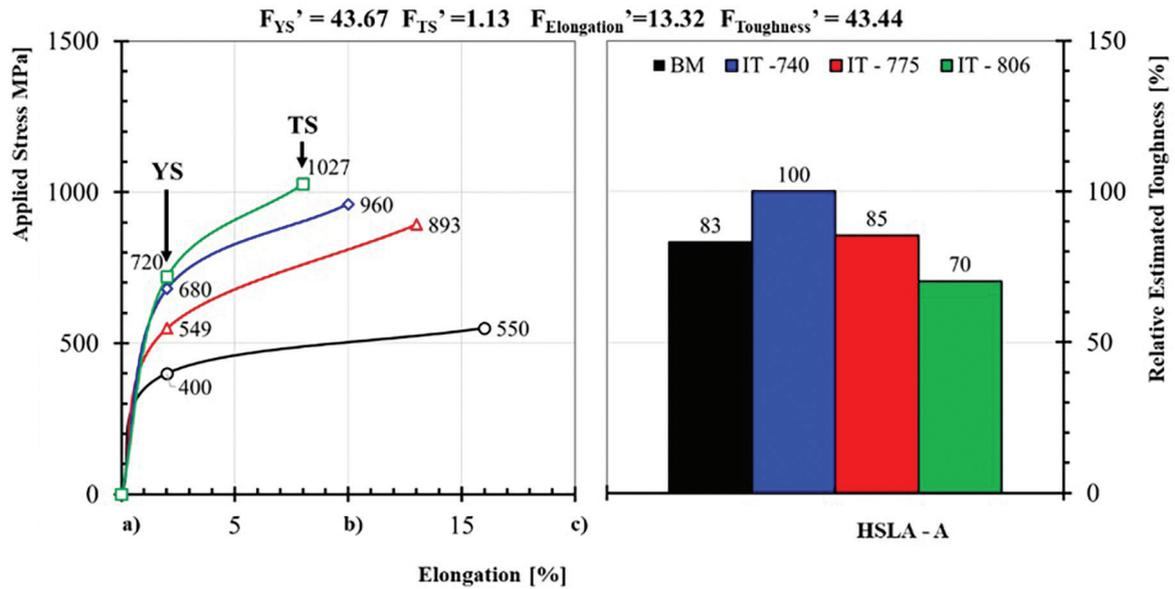
Figure 7: Mechanical properties of HSLA – A steels, prior and after quenched at three intercritical temperatures.
