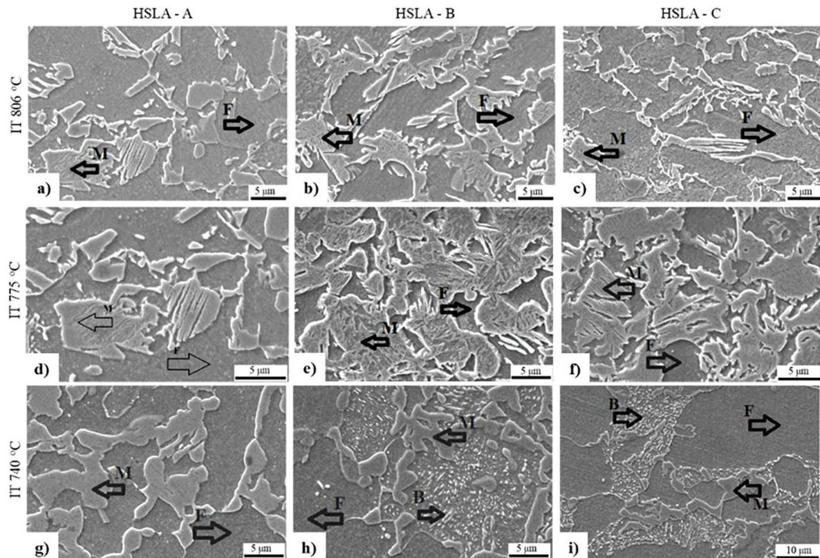
Figura 4: SEM micrographics of HSLA intercritical quenched steels.
