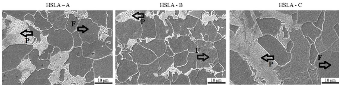
Figura 3: SEM analysis of the HSLA samples (prior to intercritical treatments).
