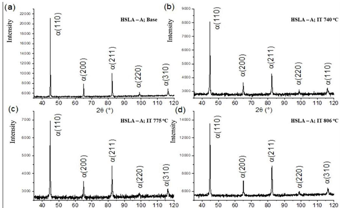
Figure 8: XRD of HSLA – A intercritical quenched steels.
