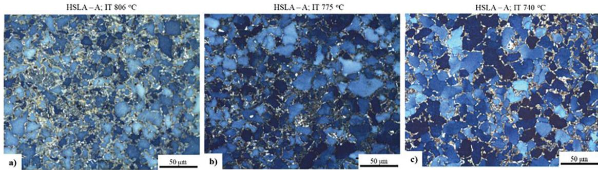
Figure 5: Microstructure of HSLA – A quenched steel, after Klemm I attack.
