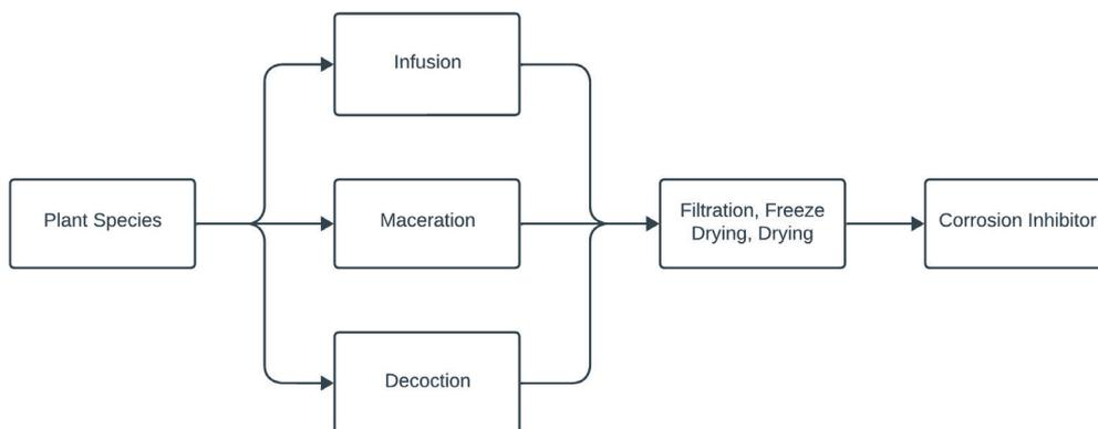
Figure 1: Methodology of obtaining a corrosion inhibitor.
