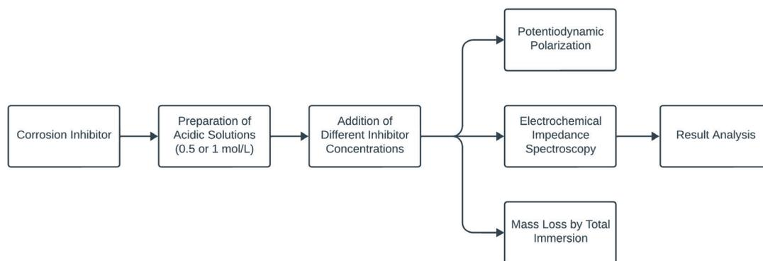
**Figure 2:** Testing procedure of corrosion inhibitors.
