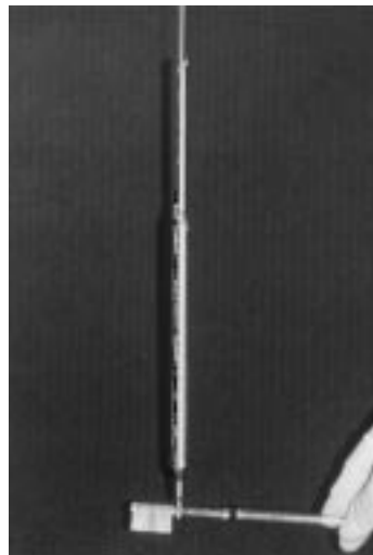
FIGURE 2 - Dinamometer coupled to the toothbrush for the standardization of the toothbrushing force in 0.2 kgf.
